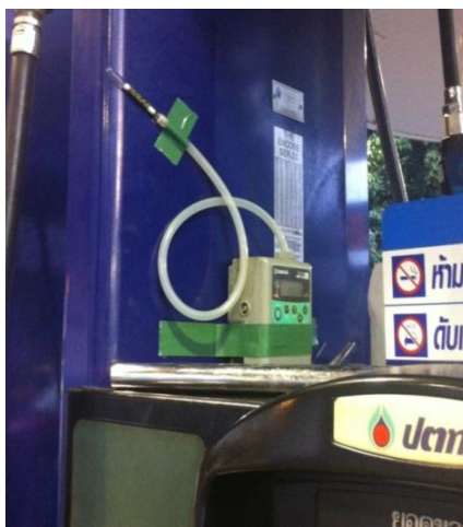
Figure 3.5 Sampling equipment for this study using a personal air pump connected with a charcoal glass tube
