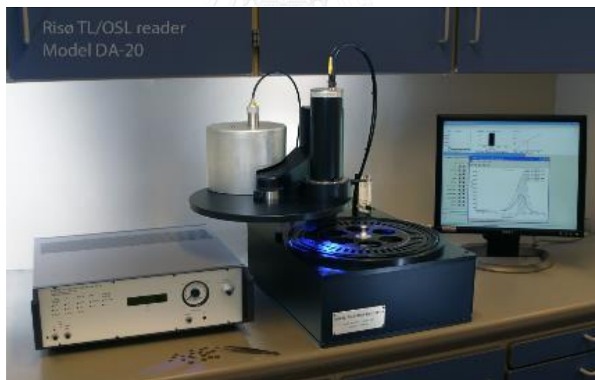
Figure 3.8 Riso TLD dosimeter at Department of Geology, Faculty of Science, Chulalongkorn University, used for OSL glow curve measurement.
