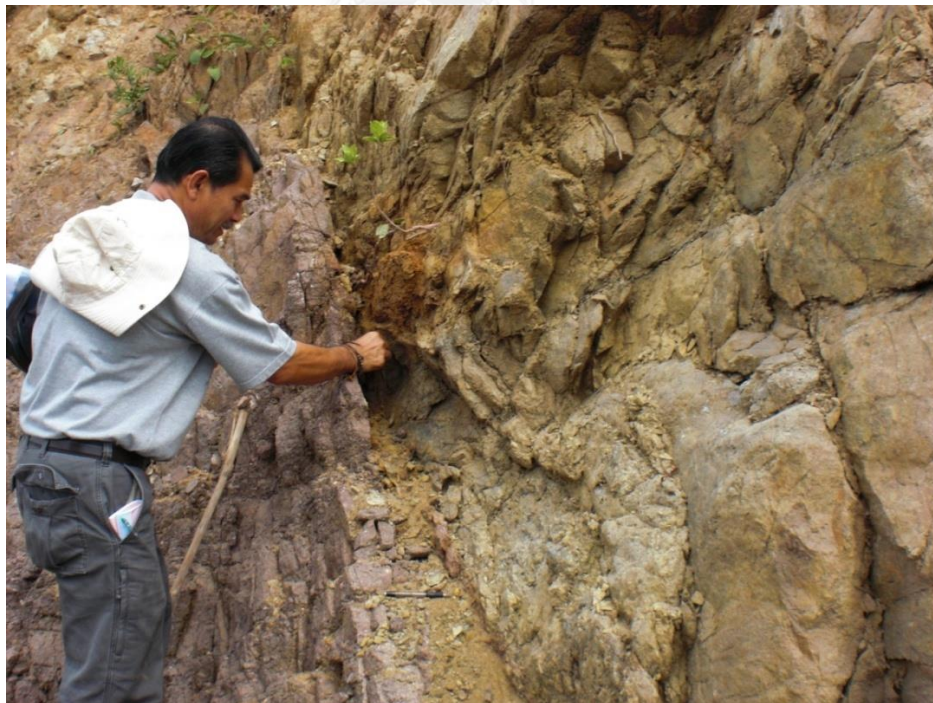
Figure 4.34 A fault gouge found along the fault plane between two sandstone (left) and siltstone (right) of the Upper Paleozoic age, Near area 4.
