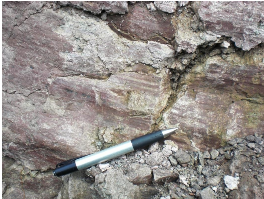
Figure 4.37 A quarry near the road near area 4 showing slickenside in the Upper Paleozoic strata, indicating a left lateral strike slip fault.
