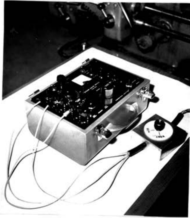
Fig. 3.9 strain gauge bridge & selector switch
