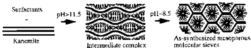
Figure 2.20 Schematic models representing “folding sheets” mechanism [56].
