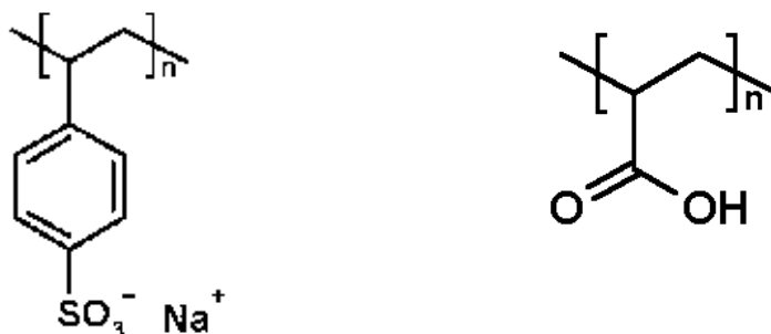
Figure 2.6 Chemical structures of two synthetic polyelectrolytes, as examples. To the left is poly(sodium styrene sulfonate) (PSS), and to the right is polyacrylic acid (PAA) [21].
