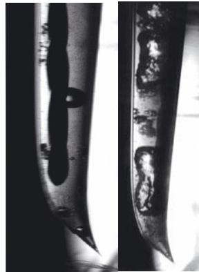
Figure 11: (left) cavitation phenomenon and streaming pattern (right) vigorous microstreaming and collapsing cavitation bubbles in glass root canal model (21)
