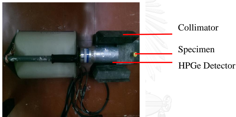
Figure 3.5: Experiment Set Up for Part I Samples with HPGe Detector
