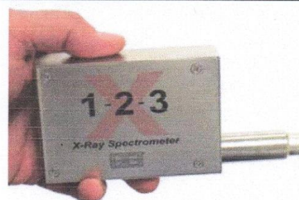
FIGURE 1. The CdTe detector in the X-123CdTe configuration
