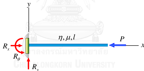
Figure 4.1 A perfectly straight nano-beam clamped at left end and subjected to longitudinal concentrated force P at the tip
