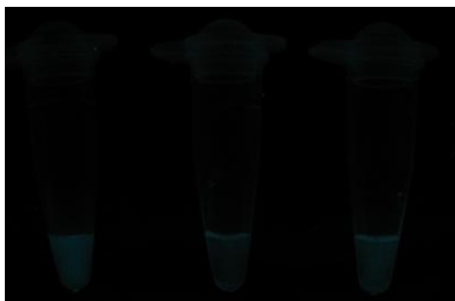
Figure 3.9 Fluorescent MBS1 photographs under black light (405 nm) (left: single stranded, middle: hybrid with complementary DNA, right: hybrid with single-base mismatched DNA). Conditions: 10 mM phosphate buffer pH 7.0, [PNA] = 10 \mu M and [DNA] = 12 \mu M.
