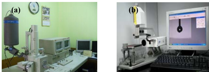
Figure 3.3 Scanning electron microscope (a) and water CA measurement (b), respectively
