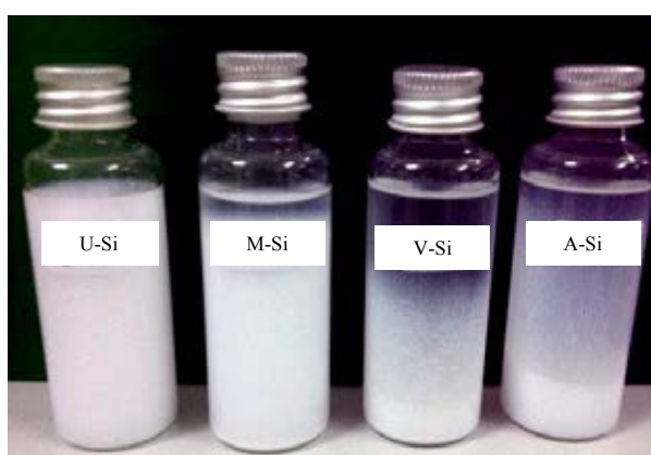
Figure 4.2 The suspension of U-Si, M-Si, V-Si and A-Si particles, respectively in ethanol (after synthesis for 1 week)
