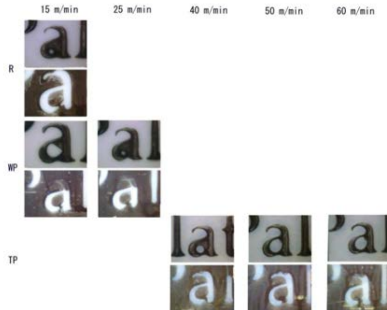
Figure 4-25 Printed positive and negative fonts of nano silver ink on 3 substrates using printing speed at 15, 25, 40, 50 and 60 m/min.
