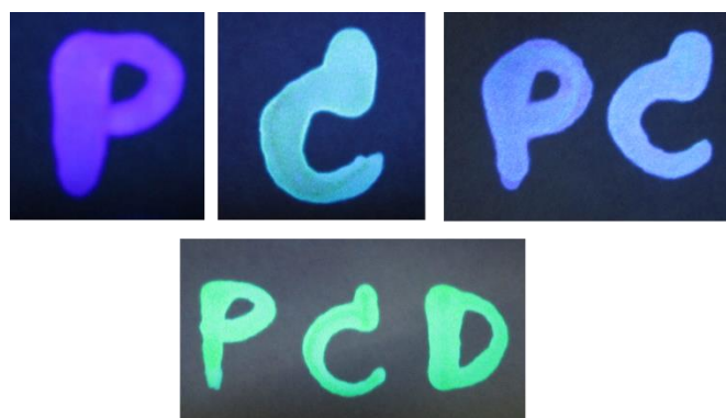
Figure 2.24 Photographs of the fluorescence images of sensor PBA ; P, sensor CA ; C, the mixture of sensors PBA and CA in the absence of DA; PC and in the presence of DA; PCD.
