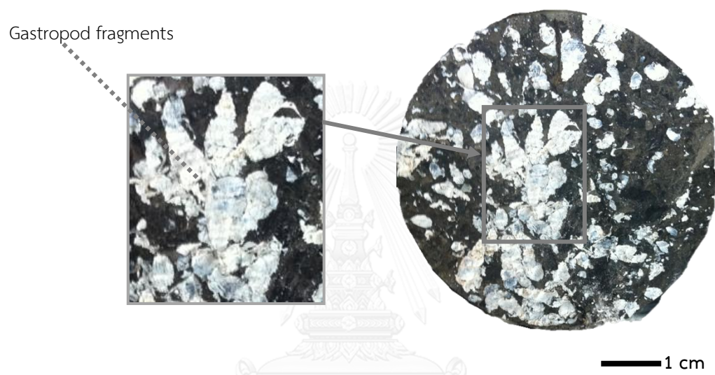
Figure 3.20 Mesoscopic of J6 subseam - brownish black to grayish black, dull, brittle, and gastropods remain ( Melanoides sp. ).
