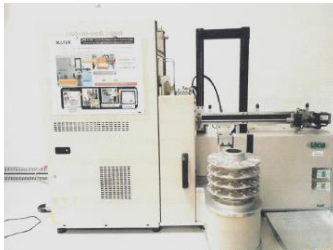
Figure 3.28 S determinator (LECO SC632) for sulphur contents at Laboratory Section, Mae Moh Mine.
