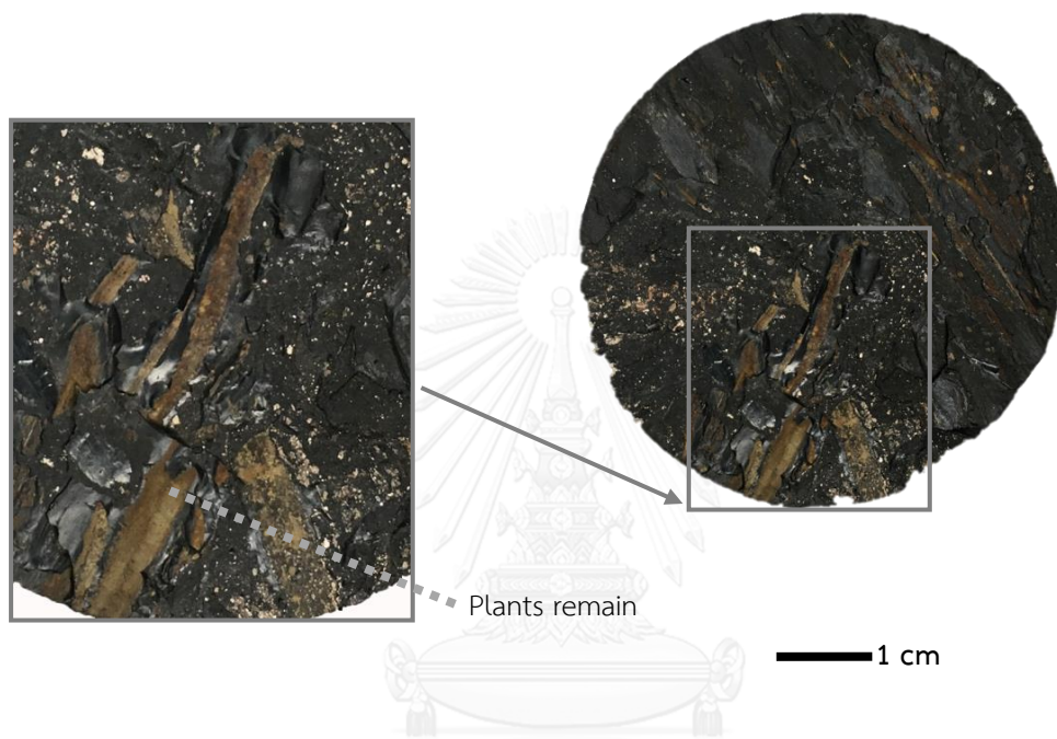
Figure 3.14 Mesoscopic of Q3 subseam - grayish black to black, dull, brittle to hard, sub-conchoidal to conchoidal fracture and plant remains.
