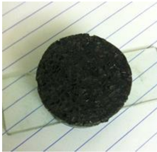
Figure 3.24 The polished section of coal for petrographic microscope study.
