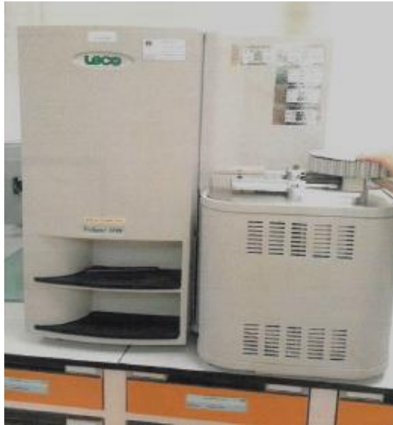
Figure 3.27 CHN determinator (LECO TRuSpec CHN) for carbon, hydrogen and nitrogen contents at Laboratory Section, Mae Moh Mine.
