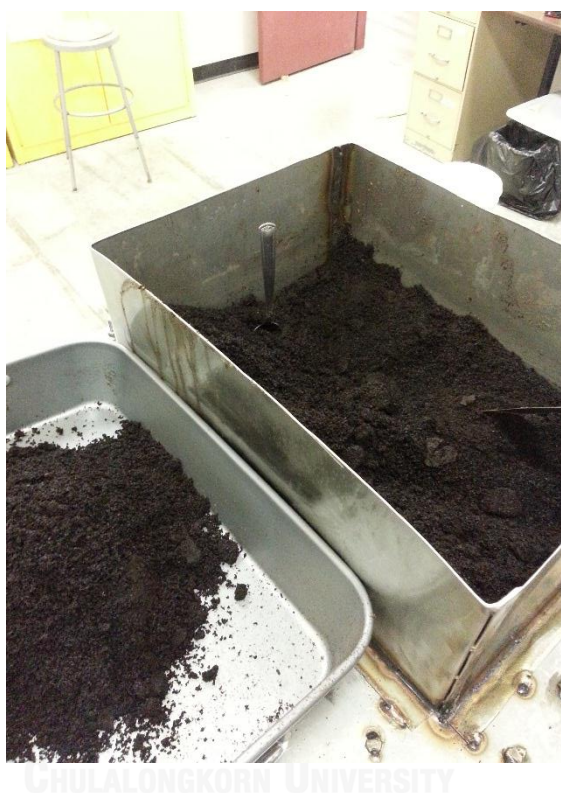
Figure C5 Separation of defatted SCG from liquid fraction after in-situ TE by paper filtration.
