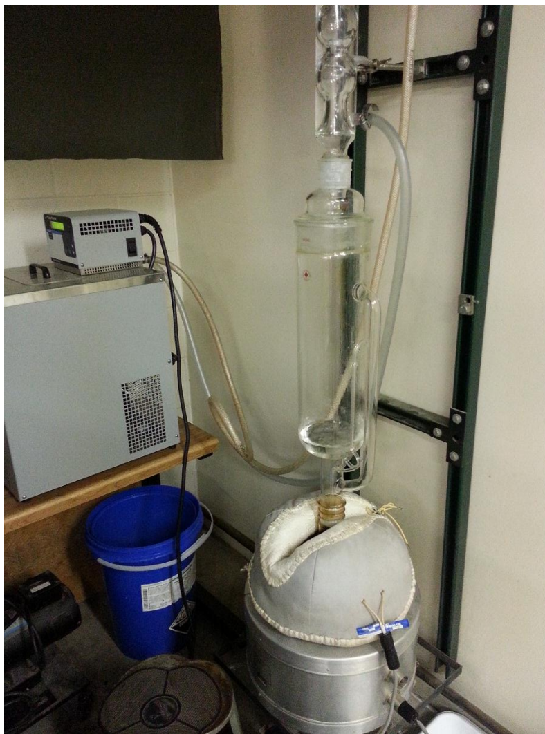
Figure C6 Methanol evaporation of liquid fraction after in-situ TE using 12 L Soxhlet apparatus.
