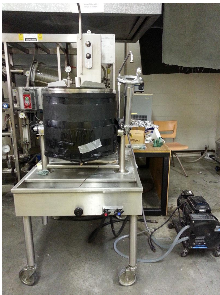
Figure C3 Pilot scale 38 L reactor used in SCG biodiesel production for processing 4 kg SCG per batch.
