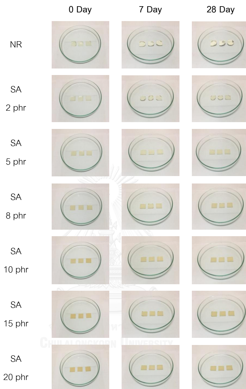
Figure A.3 The swelling behavior in water of NR-SA composite films.
