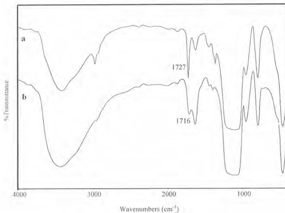
Figure 4.5 FT-IR spectra of silica particles having Pt -BA brushes (a) and PAA brushes (b)
