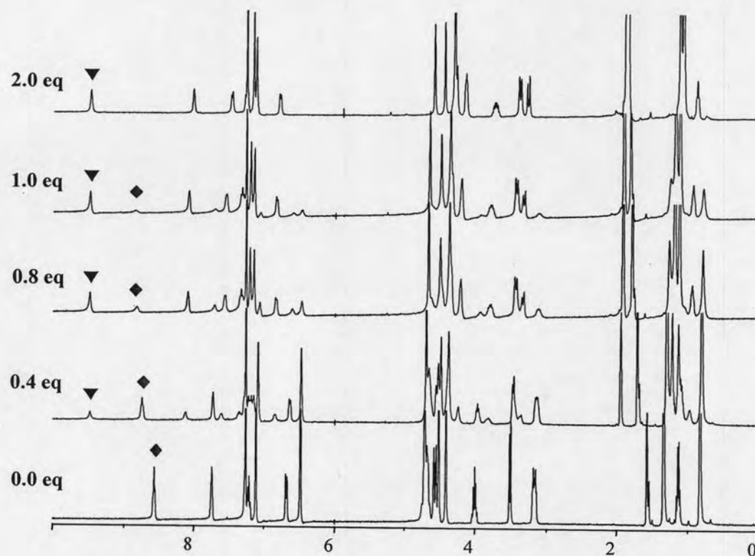
Figure A.20 ^1\text{H-NMR} titration of receptor 2 with \text{KPF}_6 in 5% \text{CD}_3\text{CN}:\text{CDCl}_3 where ▼ is NH protons of the complex [\mathbf{2}.\text{K}^+] and ◆ is NH proton of the free receptor 1
