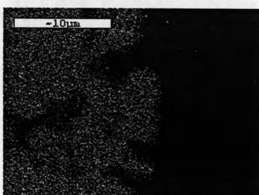
e) EDS mapping scan for nickel
