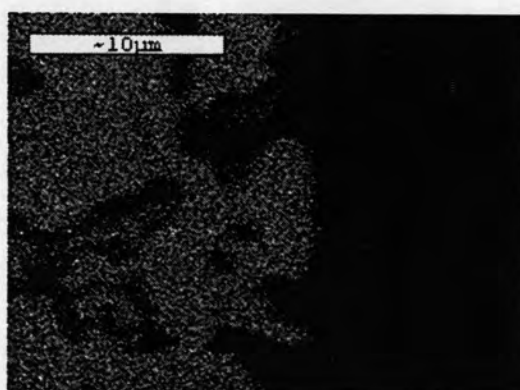
c) EDS mapping scan for iron
