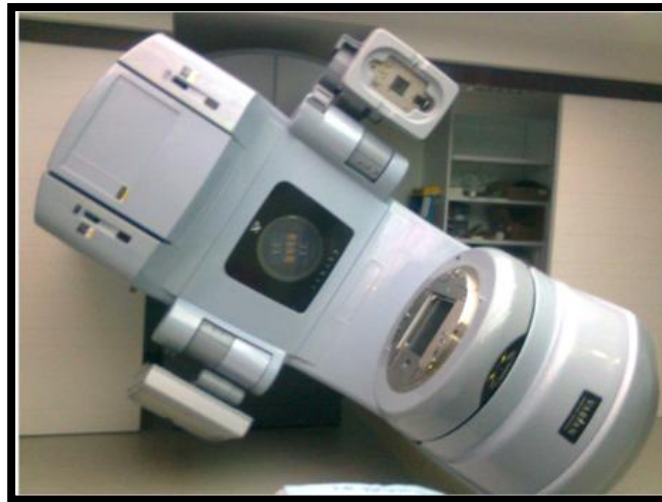
Figure 3.10 Varian Clinic iX linear accelerator (Varian Oncology systems, Palo Alto, CA, USA)
