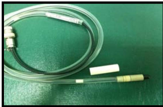
Figure 3.6 The CC13 ionization chamber (Scanditronix, Wellhofer Dosimetries, Schwarzenbruck, Germany)
