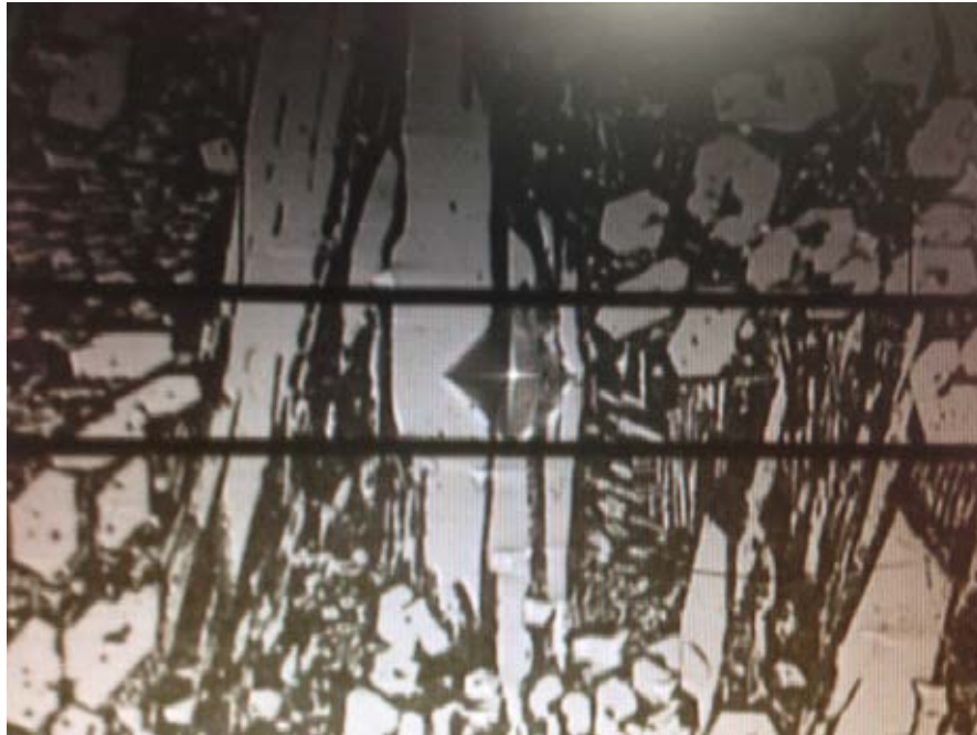
Figure 3.11 Measuring length of diamond pyramid cavity on microstructure
