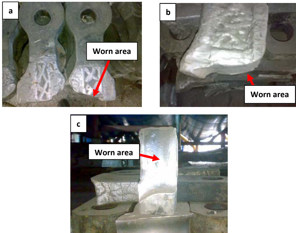
Figure 2.4 Shredder hammer after use 18 days (a) Top view (b) Side view (c) Front view
