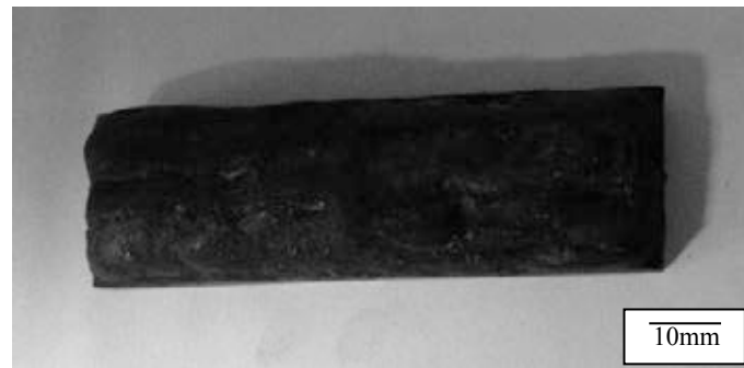
Figure 3.2 Base material after full hardfacing on the surface.
