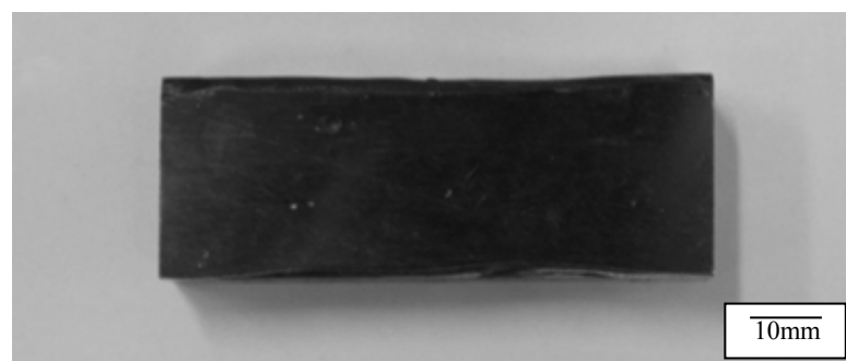
Figure 3.3 Flat surface of hardfaced samples after grinding.
