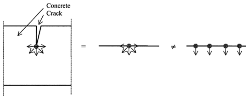
Figure 2.26. Chloride ions spread in two (three) dimension (Paulsson-Tralla and Silfwerbrand, 2002)
