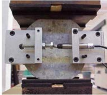
Figure 2.6. Controlled splitting test (Djerbi et al., 2008a)
