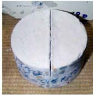
Figure 2.5. The artificial crack (notch) by Marsavina (Marsavina et al., 2009)
