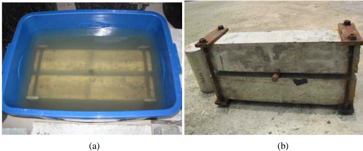
Figure 5.21. Immersion (a) and after immersion (b) of cracked beam in salt solution
