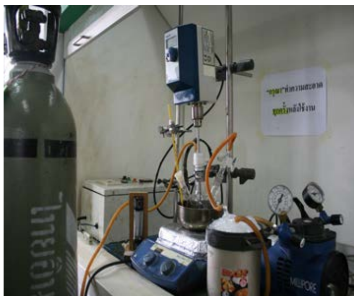
Figure 4.1 Experimental setup for melt transesterification of DPC and BPA.
