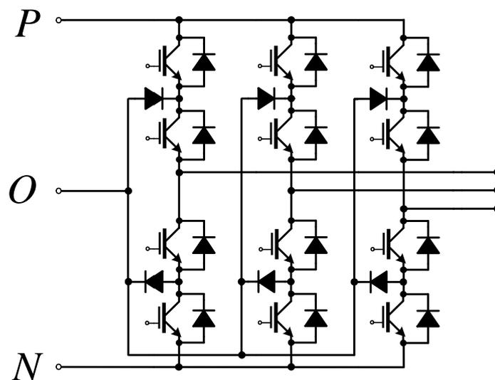
Figure 3.2 Three-phase three-level NPC structure.
