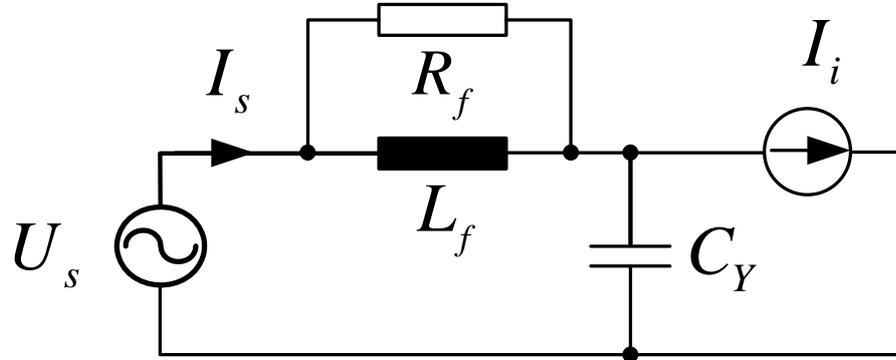
Figure 5.4 Simple per-phase equivalent circuit used for filter design
