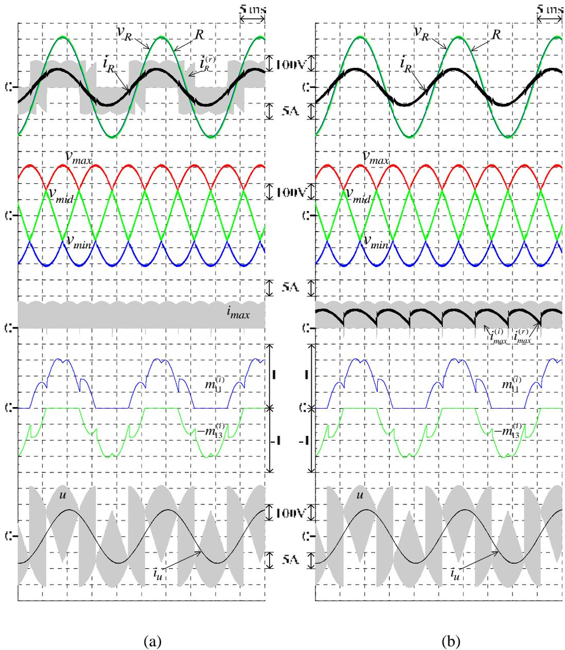
Figure 4.19 External and internal waveforms of the proposed 3L-BTB converters with leading input power factor ( $M = 0.7$ ,  $f_o = 50$  Hz,  $k_1 = -3.3$ ) (a) 3L-IMC (b) S3L-BTB converter
