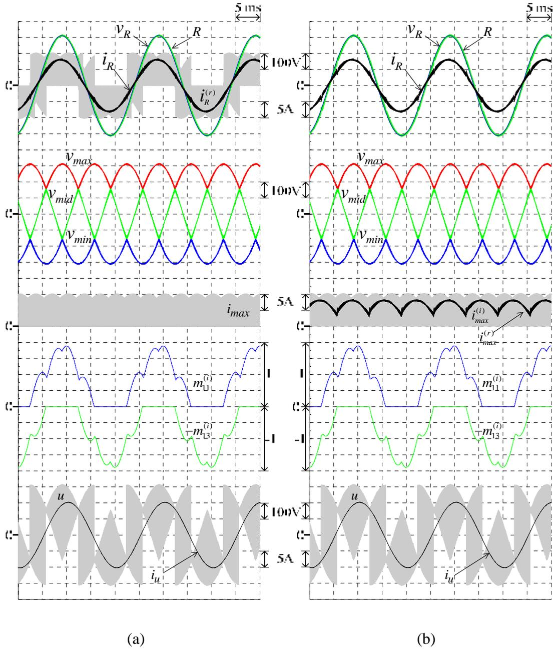
Figure 4.7 External and internal waveforms of the proposed 3L-BTB converters under output voltage variation ( $M = 0.86$ ,  $f_o = 50$  Hz) (a) 3L-IMC (b) S3L-BTB converter
