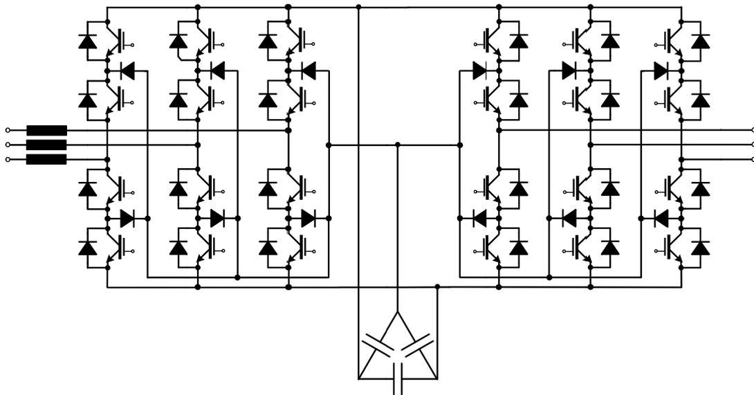
Figure 3.4 Symmetrical three-level back-to-back converter (S3L-BTB converter).
