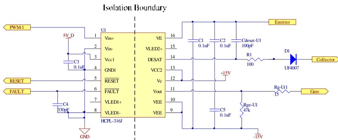
Figure 5.3 Schematic of a gate drive circuit.
