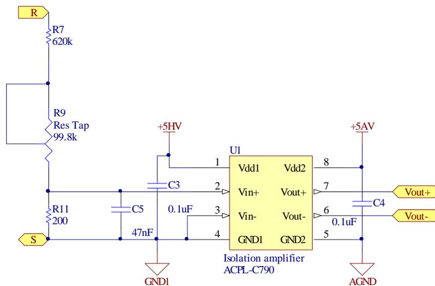
Figure 5.7 Schematic of the line-to-line voltage sensing circuit.
