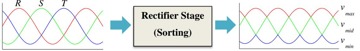
Figure 2.3 Sorting operation of the rectifier stage
