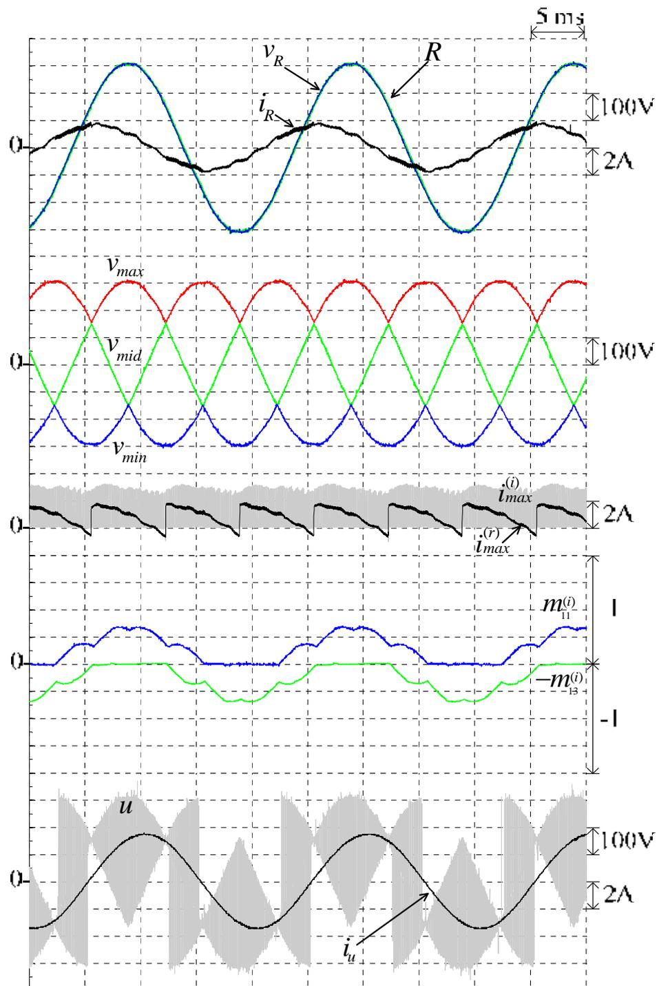
Figure 5.14 Measured waveforms of the prototyped S3L-BTB converter under output voltage variation at  $(M = 0.3, f_o = 50 \text{ Hz})$
