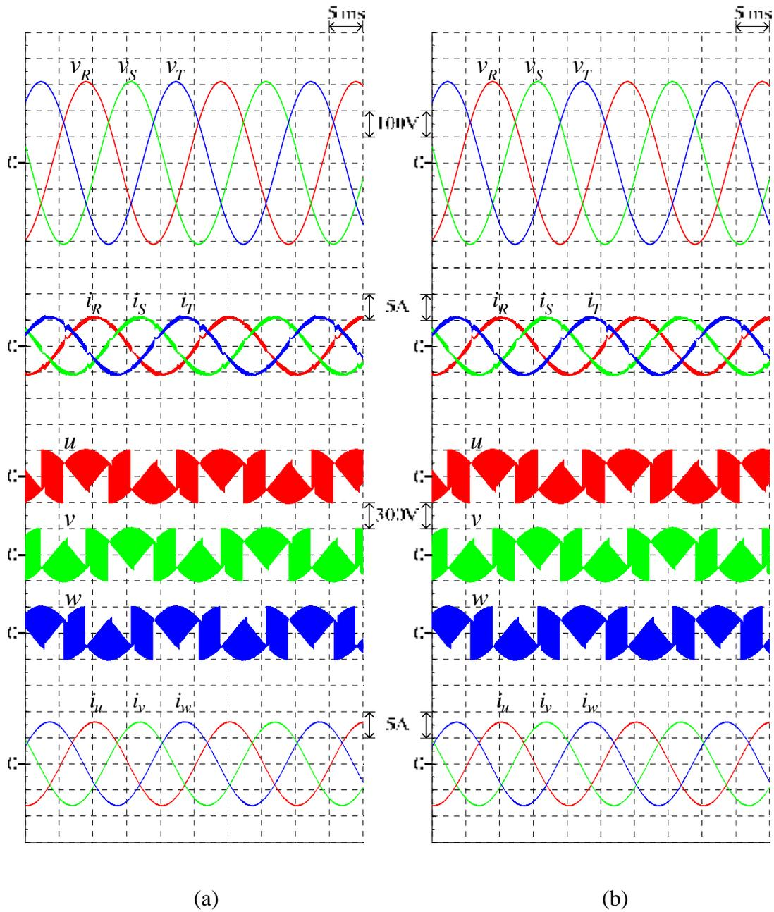
Figure 4.16 Simulated input-output waveforms of the proposed 3L-BTB converters with lagging input power factor ( $M = 0.7$ ,  $f_o = 50$  Hz,  $k_1 = 15$ ) (a) 3L-IMC (b) S3L-BTB converter
