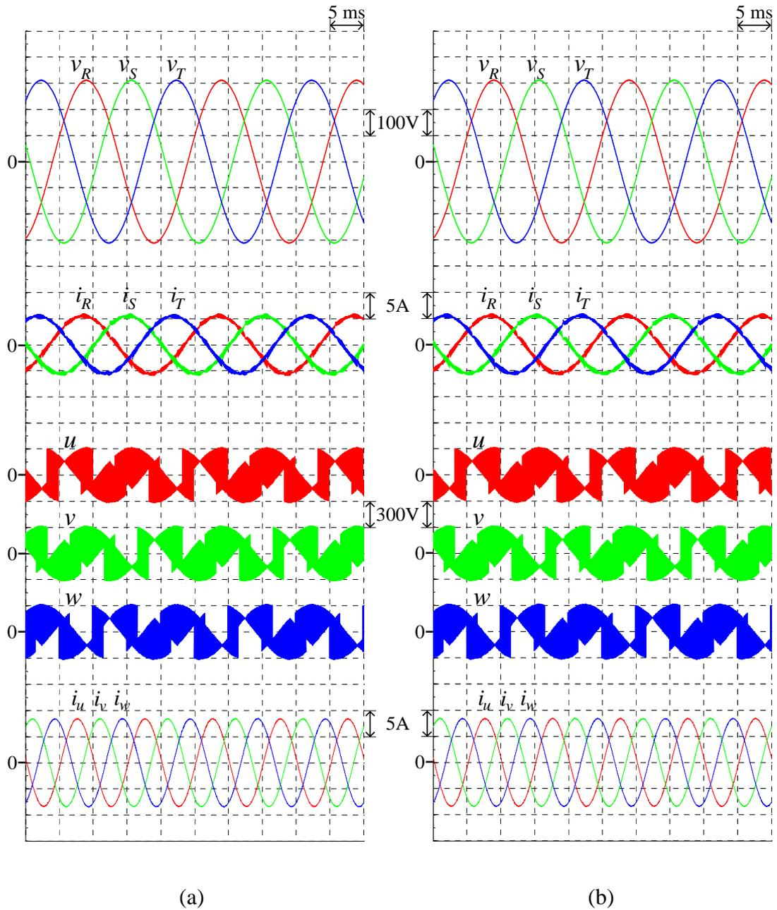
Figure 4.10 Simulated input-output waveforms of the proposed 3L-BTB converters under output frequency variation ( $M = 0.86$ ,  $f_o = 100$  Hz) (a) 3L-IMC (b) S3L-BTB converter
