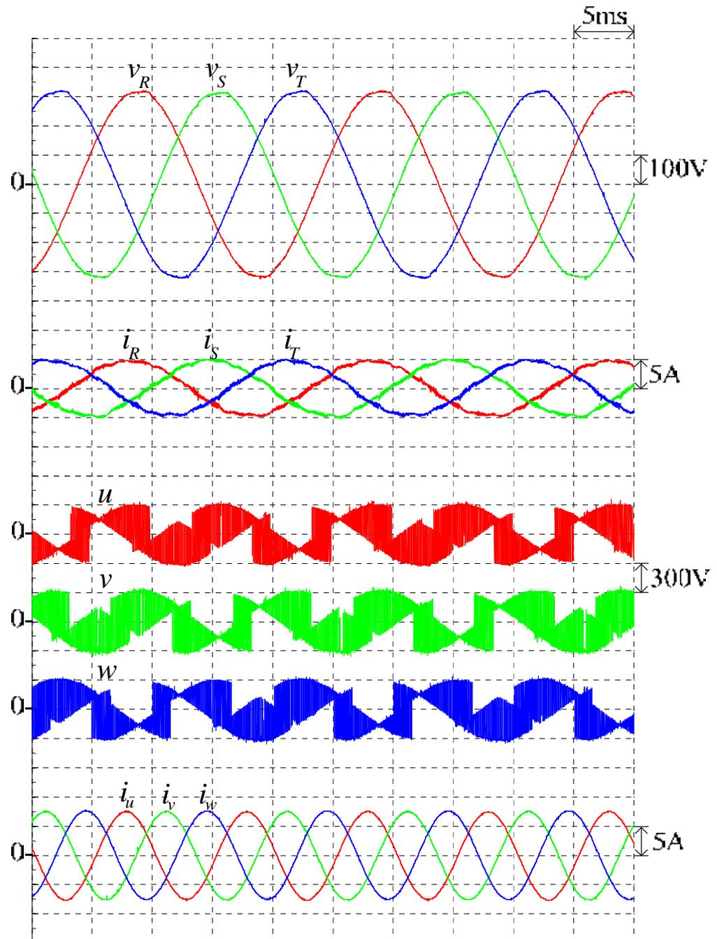
Figure 5.21 Measured input-output waveforms of the prototyped S3L-BTB converter under output frequency variation at ( $M = 0.86, f_o = 100$  Hz)
