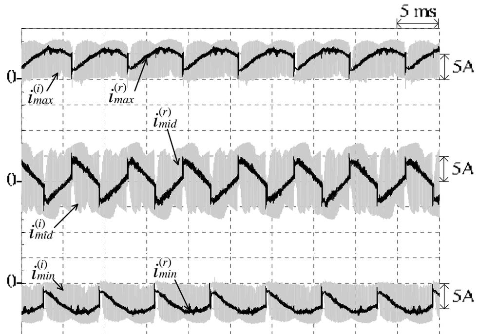
Figure 5.33 Measured dc-link current waveforms of the prototyped S3L-BTB converter with lagging input power factor compensation at ( $M = 0.7, f_o = 50$  Hz,  $k_1 = 15$ )
