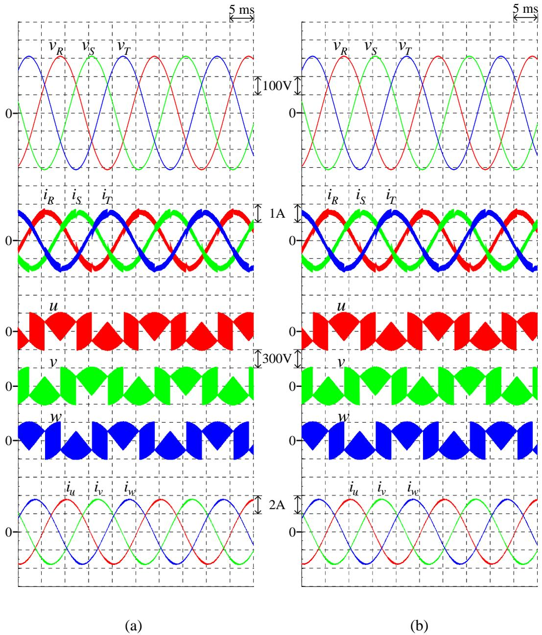
Figure 4.4 Simulated input-output waveforms of the proposed 3L-BTB converters under output voltage variation ( $M = 0.3$ ,  $f_o = 50$  Hz) (a) 3L-IMC (b) S3L-BTB converter
