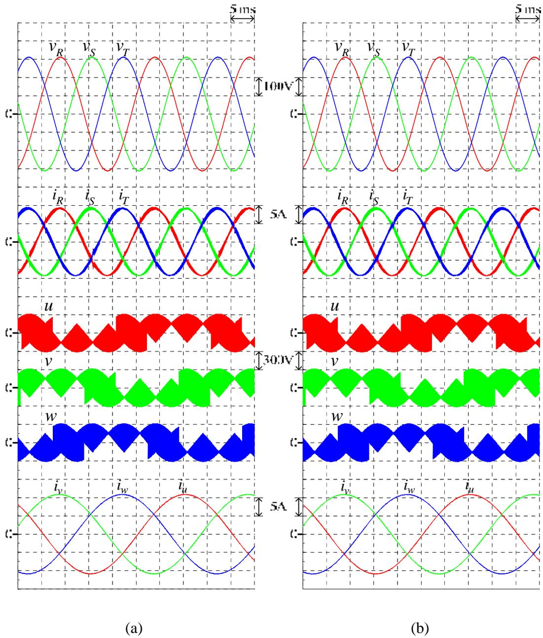
Figure 4.8 Simulated input-output waveforms of the proposed 3L-BTB converters under output frequency variation ( $M = 0.86$ ,  $f_o = 25$  Hz) (a) 3L-IMC (b) S3L-BTB converter
