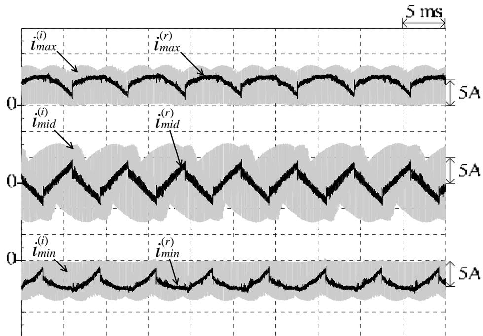
Figure 5.31 Measured dc-link current waveforms of the prototyped S3L-BTB converter without input power factor compensation at ( $M = 0.7, f_o = 50 \text{ Hz}, k_1 = 0$ )
