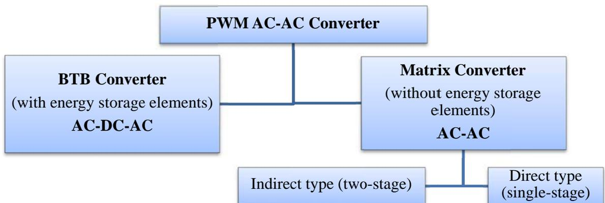
Figure 1.1 Classification of three-phase PWM AC-AC converters.
