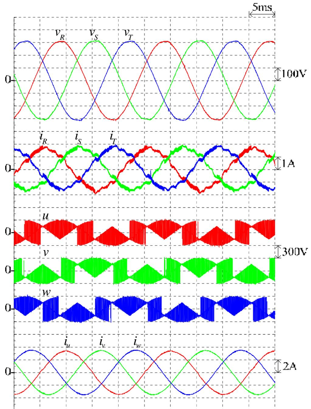
Figure 5.13 Measured input-output waveforms of the prototyped S3L-BTB converter under output voltage variation at ( $M = 0.3, f_o = 50$  Hz)
