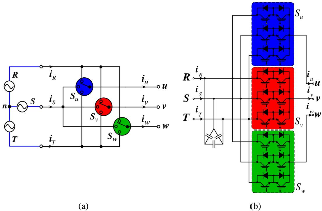
Figure 2.1 Matrix converters. (a) conceptual model (b) conventional matrix converter
