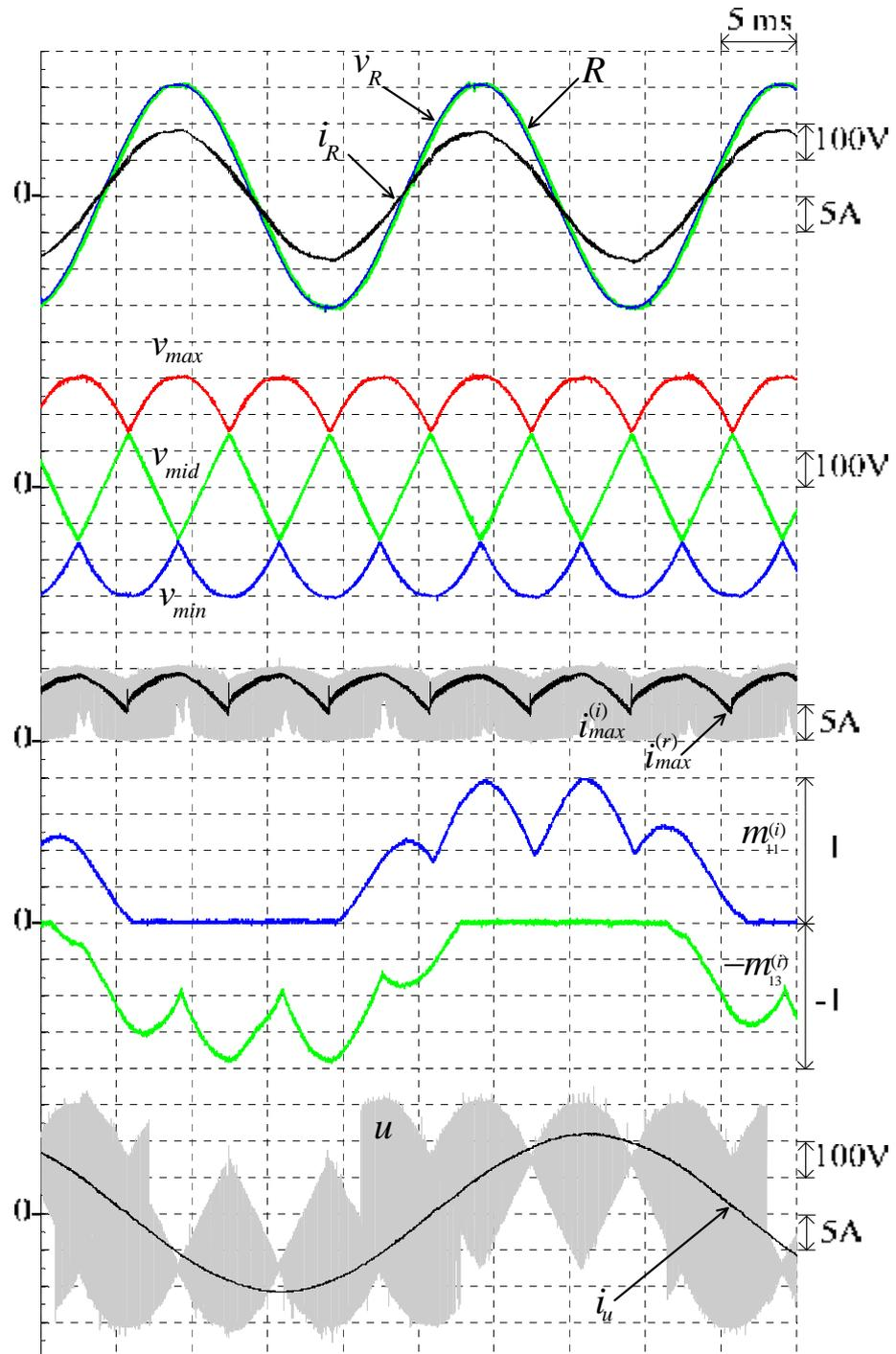
Figure 5.20 Measured waveforms of the prototyped S3L-BTB converter under output frequency variation at  $(M = 0.86, f_o = 25 \text{ Hz})$
