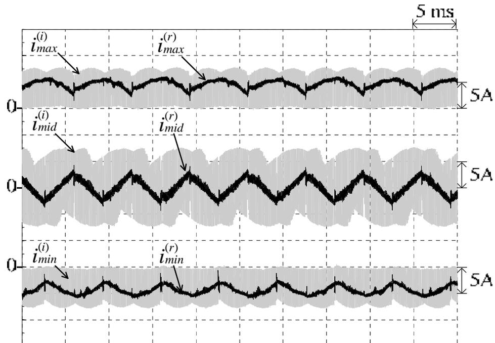
Figure 5.32 Measured dc-link current waveforms of the prototyped S3L-BTB converter with unity input power factor compensation at ( $M = 0.7, f_o = 50 \text{ Hz}, k_1 = -3.3$ )
