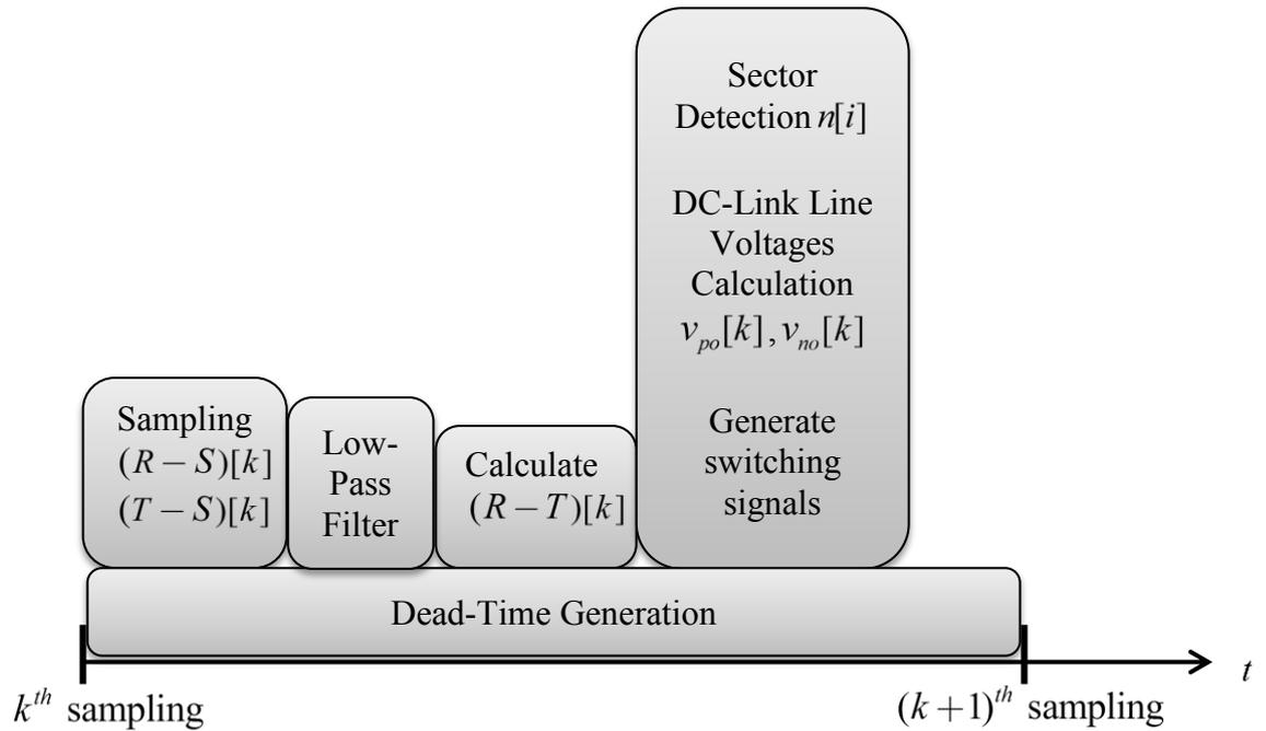
Figure 5.9 Timing diagram of the rectifier operation implemented on the FPGA. (The length of the boxes does not represent the actual time interval being used.)
