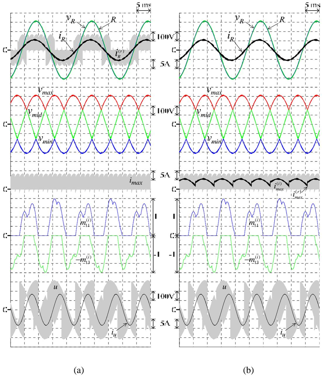
Figure 4.11 External and internal waveforms of the proposed 3L-BTB converters under output frequency variation ( $M = 0.86$ ,  $f_o = 100$  Hz) (a) 3L-IMC (b) S3L-BTB converter
