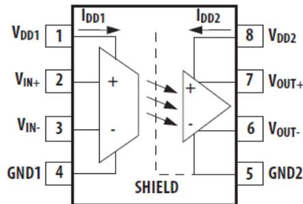
Figure 5.6 Schematic of the optical-isolation amplifier ACPL-C790C.
