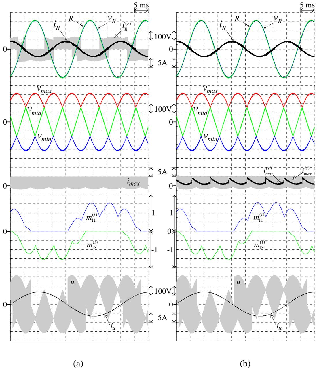
Figure 4.25 External and internal waveforms of the proposed 3L-BTB converters operating under regenerative mode ( $M = 0.7$ ,  $f_o = 25$  Hz,  $k_1 = 0$ ) (a) 3L-IMC (b) S3L-BTB converter
