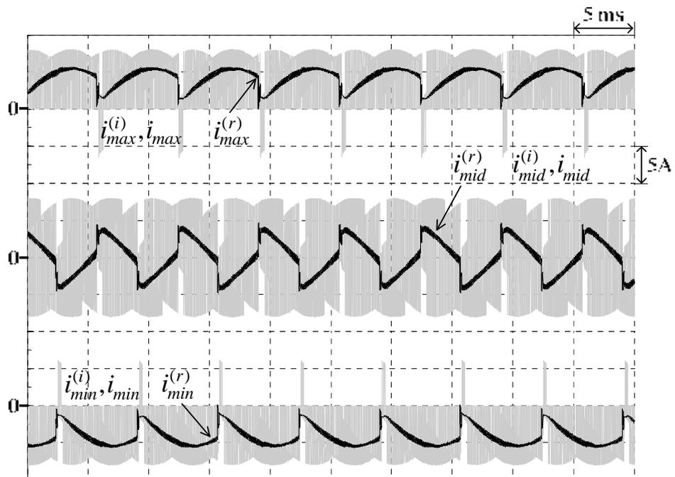
Figure 4.22 Simulated dc-link currents of the proposed 3L-BTB converters with lagging input power factor under condition ( $M = 0.7, f_o = 50 \text{ Hz}, k_1 = 15$ )
