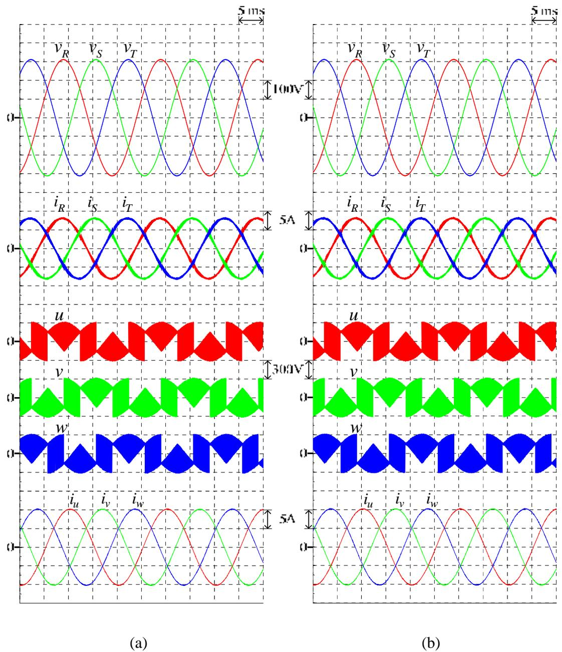
Figure 4.6 Simulated input-output waveforms of the proposed 3L-BTB converters under output voltage variation ( $M = 0.86$ ,  $f_o = 50\text{Hz}$ ) (a) 3L-IMC (b) S3L-BTB converter
