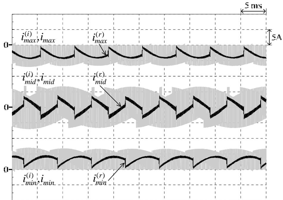
Figure 4.28 Simulated dc-link currents of the proposed 3L-BTB converters operating under regenerative mode at ( $M = 0.7, f_o = 25 \text{ Hz}, k_1 = 0$ )
