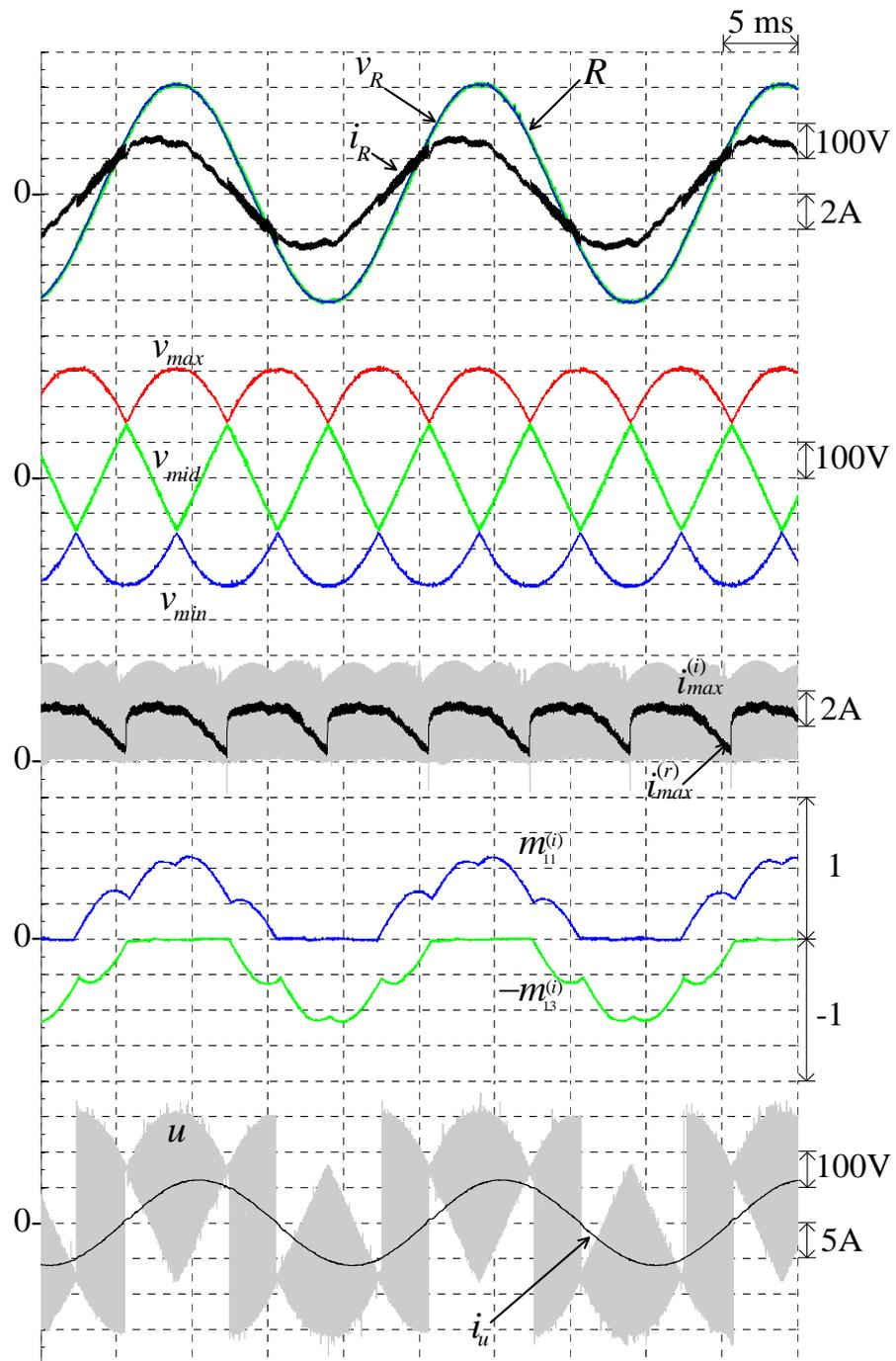
Figure 5.16 Measured waveforms of the prototyped S3L-BTB converter under output voltage variation at ( $M = 0.5, f_o = 50$  Hz)
