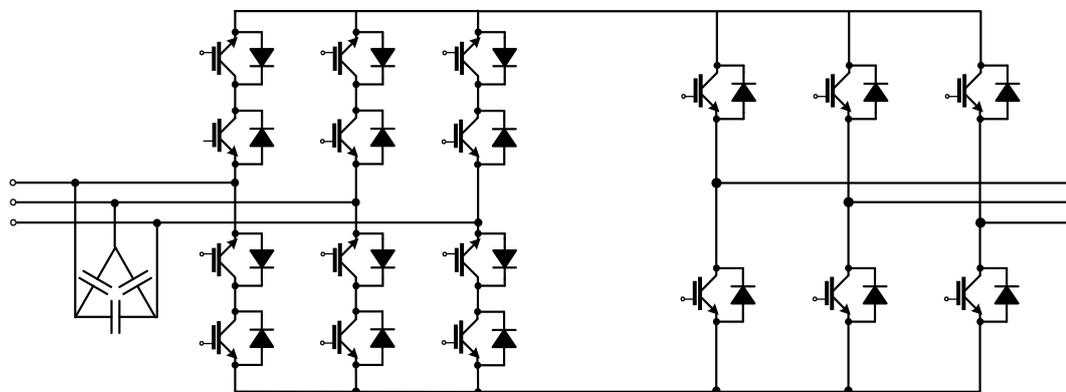
Figure 1.3 The indirect matrix converter topology
