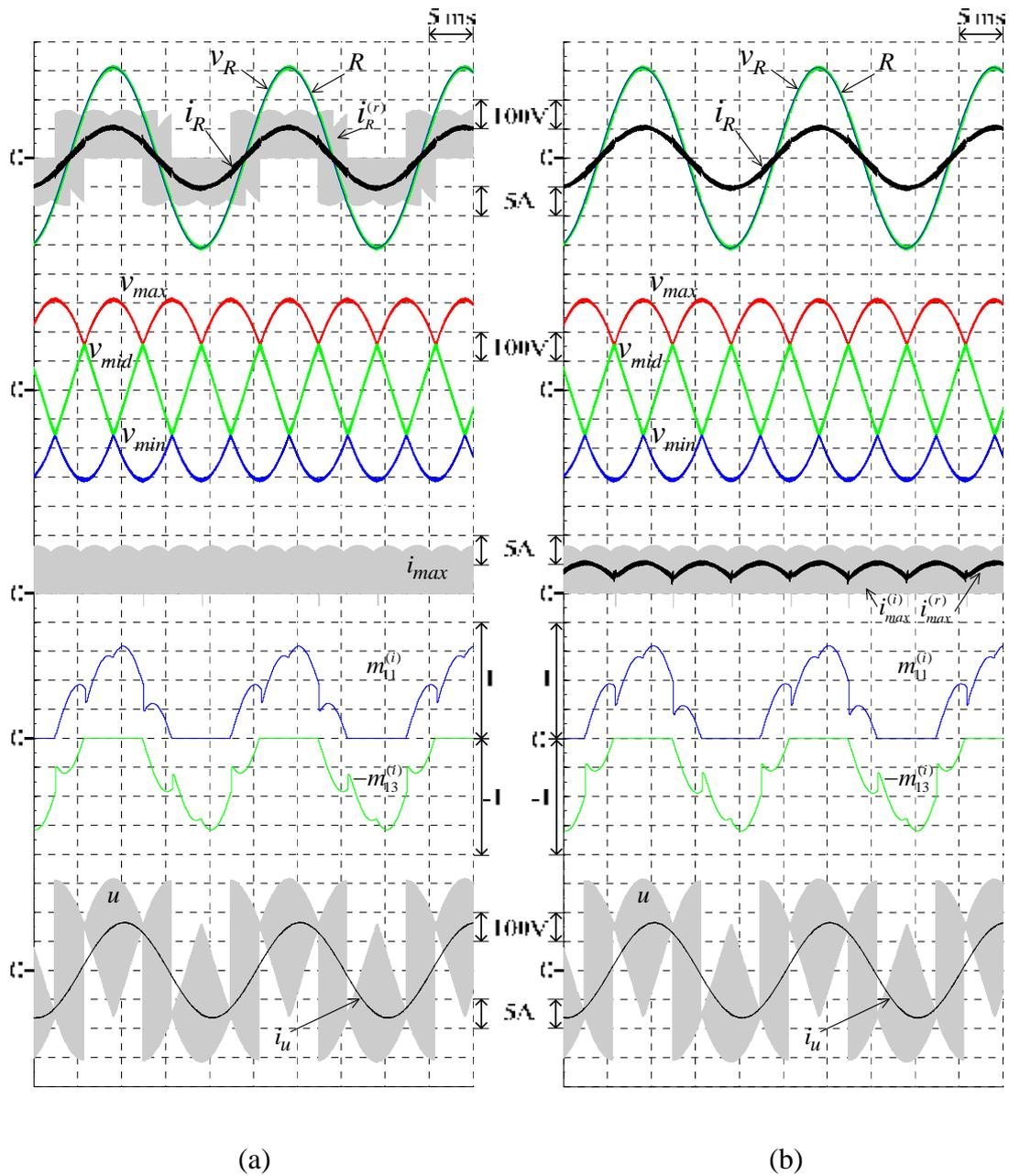
Figure 4.15 External and internal waveforms of the proposed 3L-BTB converters with unity input power factor ( $M = 0.7$ ,  $f_o = 50$  Hz,  $k_1 = 5$ ) (a) 3L-IMC (b) S3L-BTB converter
