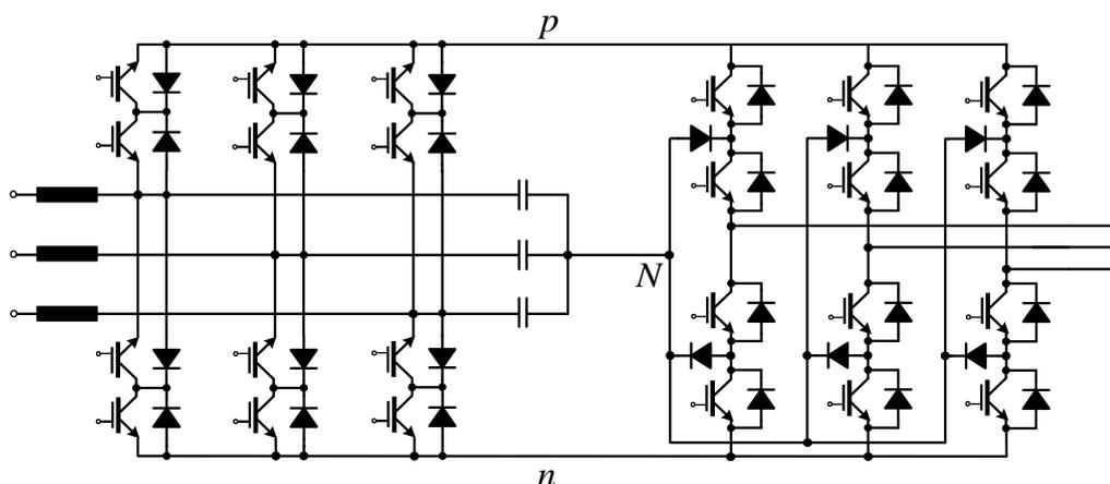
Figure 1.4 The indirect matrix converter with three-level output stage topology.
