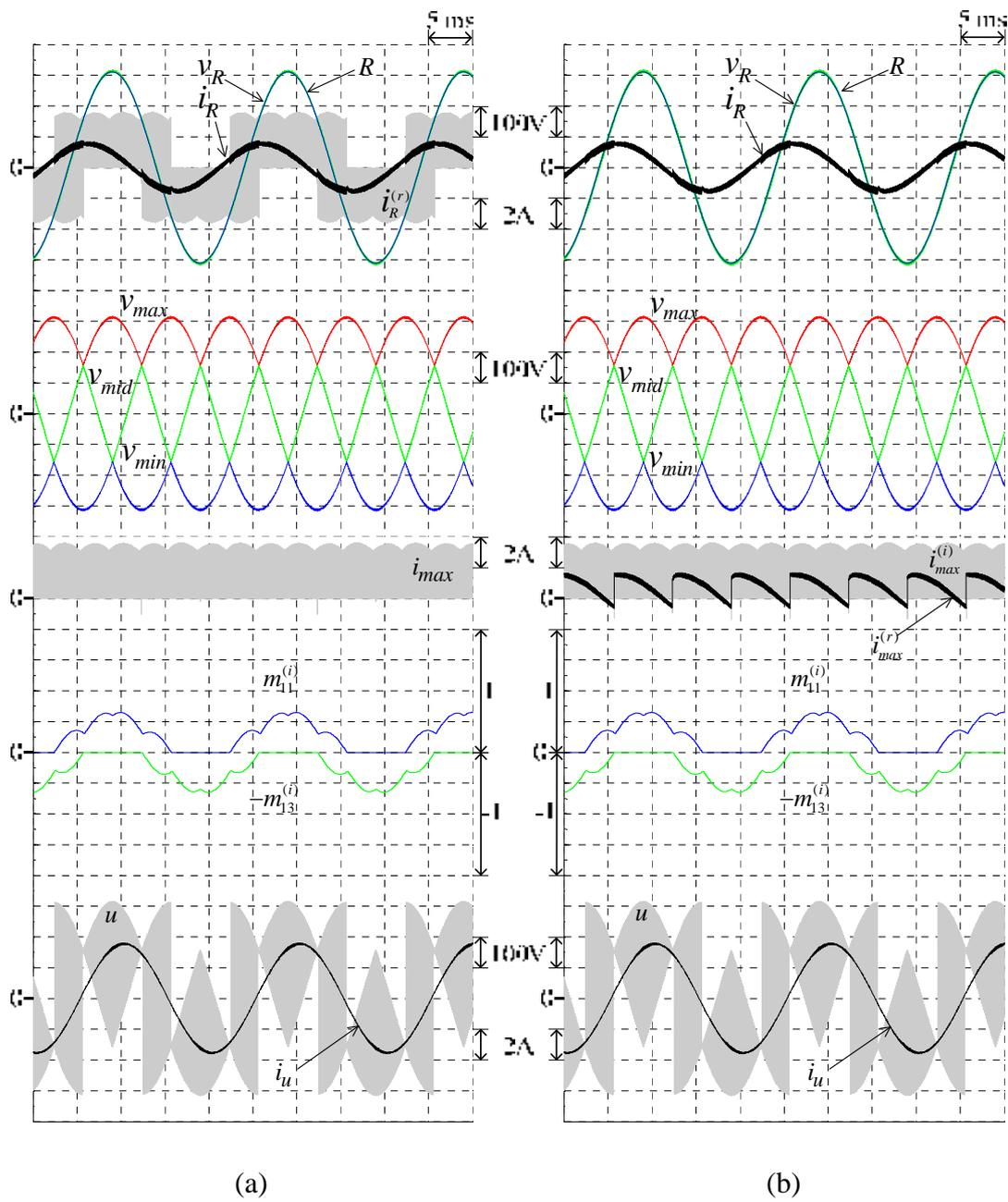
Figure 4.5 External and internal waveforms of the proposed 3L-BTB converters under output voltage variation ( $M = 0.3$ ,  $f_o = 50$  Hz) (a) 3L-IMC (b) S3L-BTB converter
