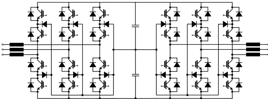
Figure 1.2 Conventional three-level back-to-back converter topology.
