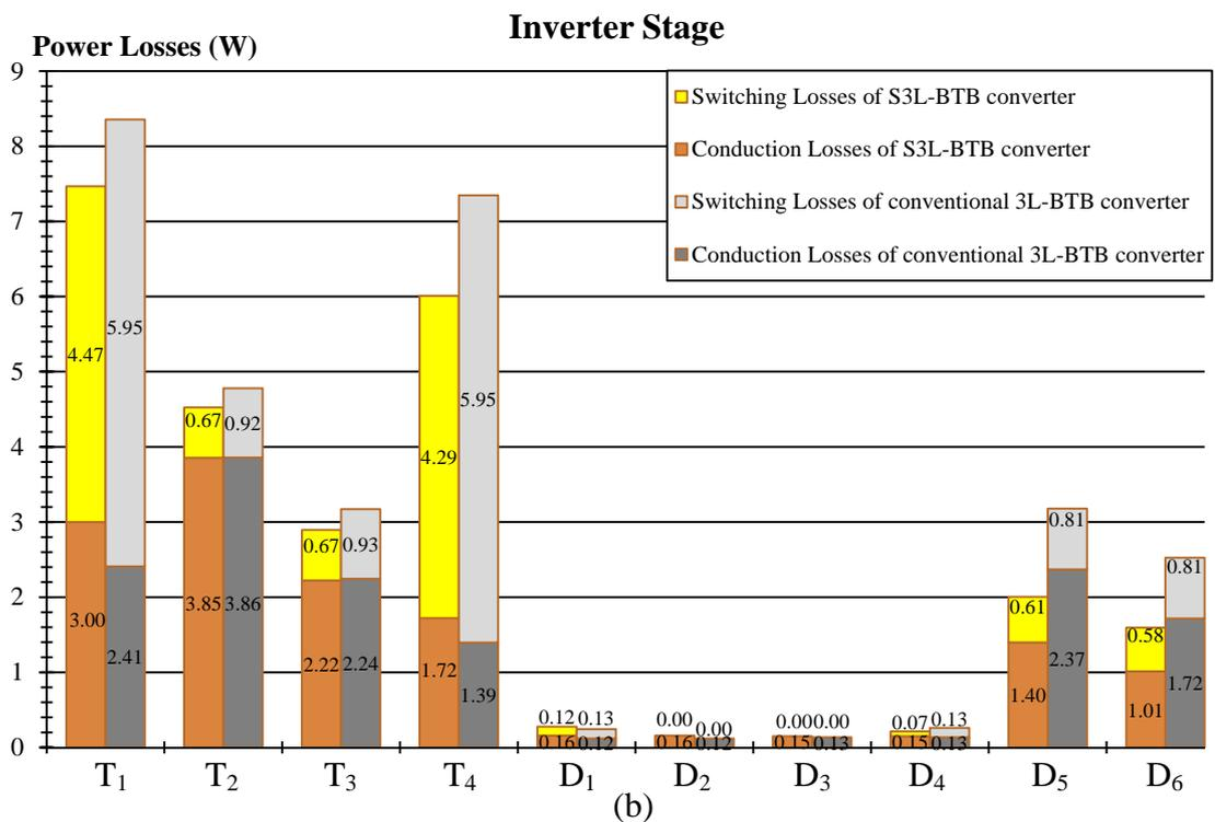
Figure 4.31 Comparison of the mean semiconductor losses between S3L-BTB and conventional 3L-BTB converters operating under condition ( $M = 0.86$ ,  $f_o = 25$  Hz)
