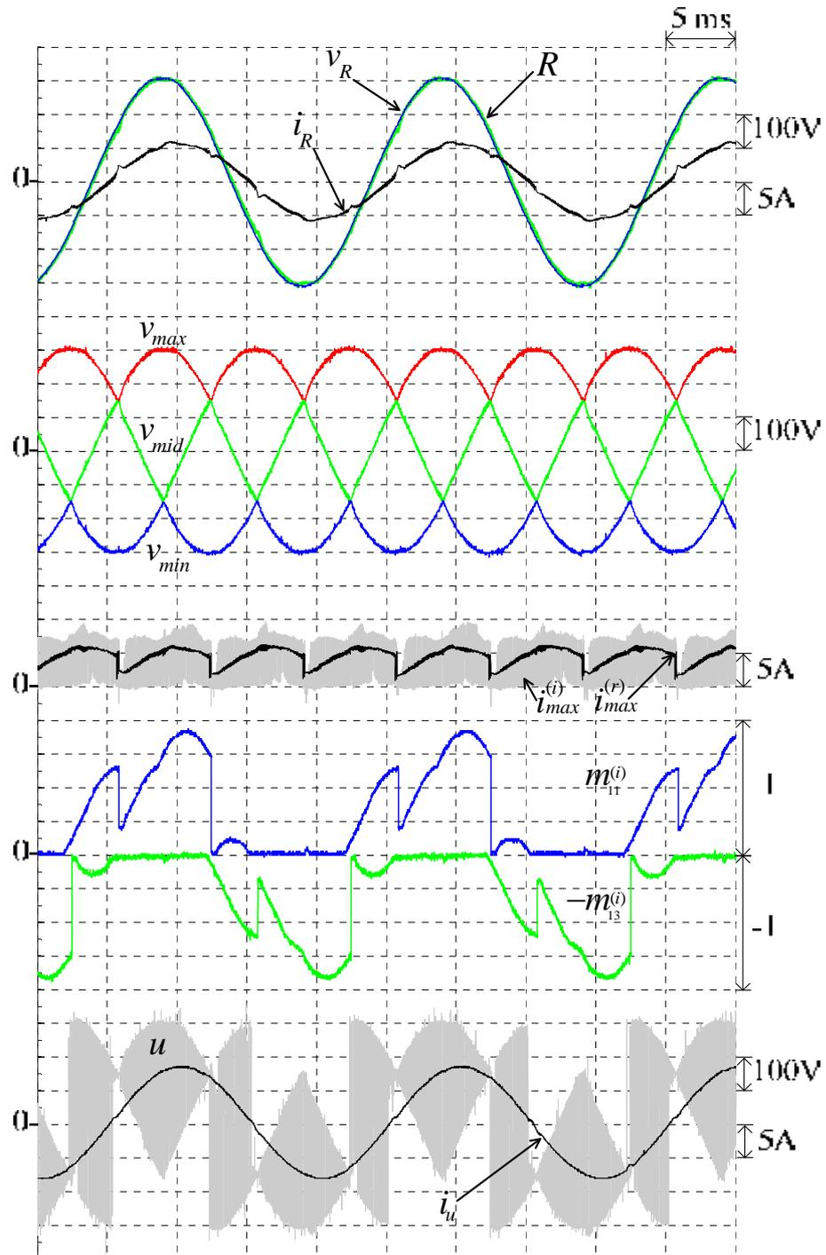
Figure 5.28 Measured waveforms of the prototyped S3L-BTB converter with lagging input power factor compensation at ( $M = 0.7, f_o = 50 \text{ Hz}, k_1 = 15$ )
