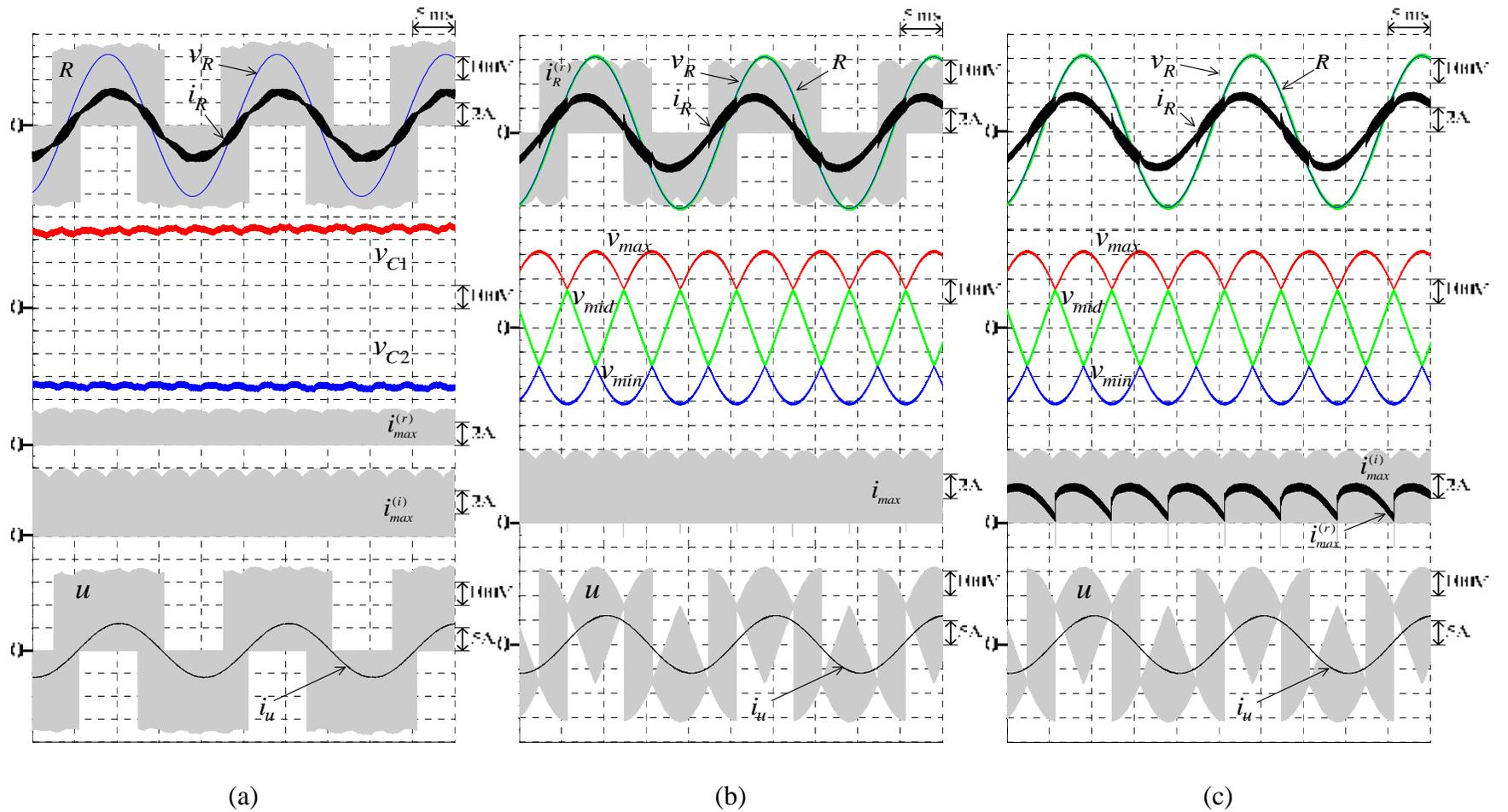
Figure 4.3 External and internal waveforms of the 3L-BTB converters working under condition 1 ( $M = 0.5, f_o = 50$  Hz)
