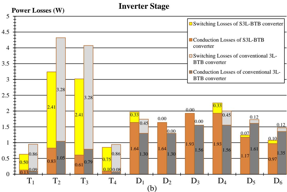
Figure 4.32 Comparison of the mean semiconductor losses between S3L-BTB and conventional 3L-BTB converters operating at unity input power factor under regenerative mode at condition ( $M = 0.7, f_o = 25$  Hz) (a) rectifier stage (b) inverter stage
