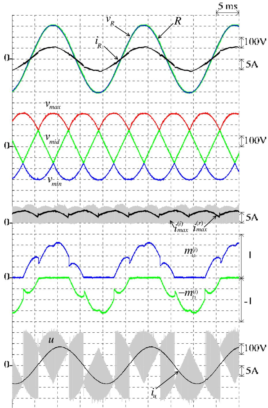
Figure 5.26 Measured waveforms of the prototype S3L-BTB converter with unity input power factor compensation at ( $M = 0.7, f_o = 50 \text{ Hz}, k_1 = 5$ )
