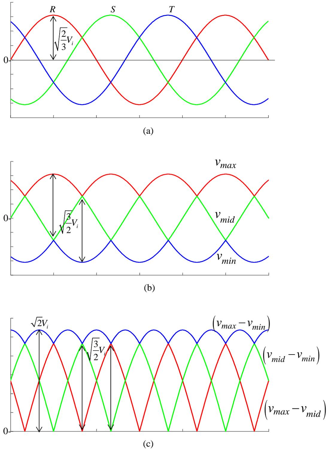
Figure 5.2 Voltages in S3L-BTB converters displayed with their peaks value
