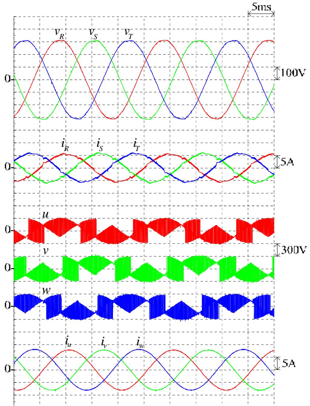
Figure 5.27 Measured input-output waveforms of the prototyped S3L-BTB converter with lagging input power factor compensation at ( $M = 0.7$ ,  $f_o = 50$  Hz,  $k_1 = 15$ )
