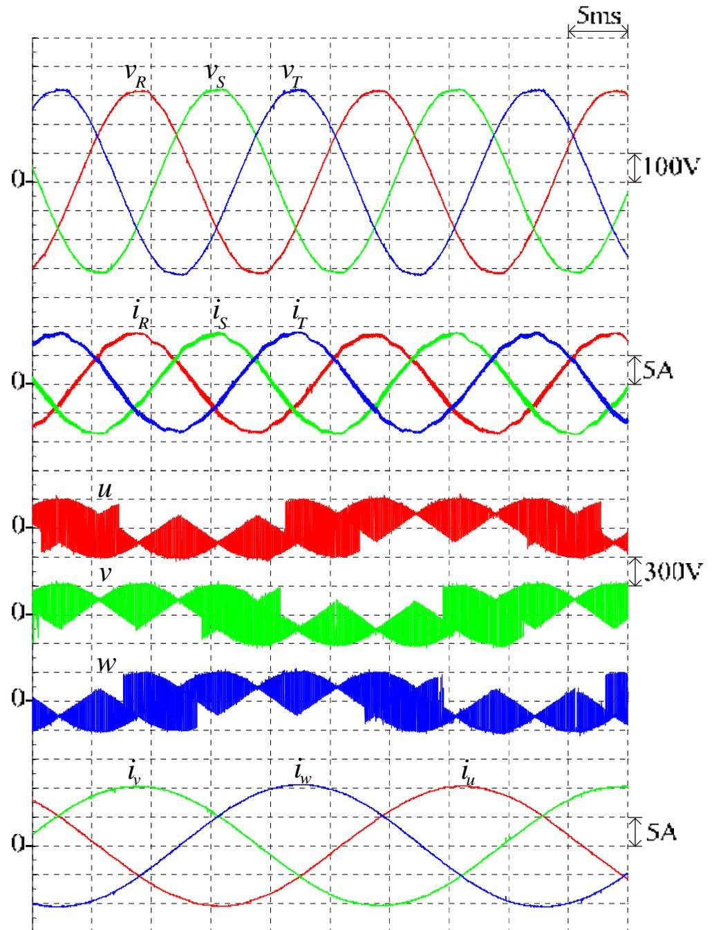
Figure 5.19 Measured input-output waveforms of the prototyped S3L-BTB converter under output frequency variation at ( $M = 0.86, f_o = 25$  Hz)
