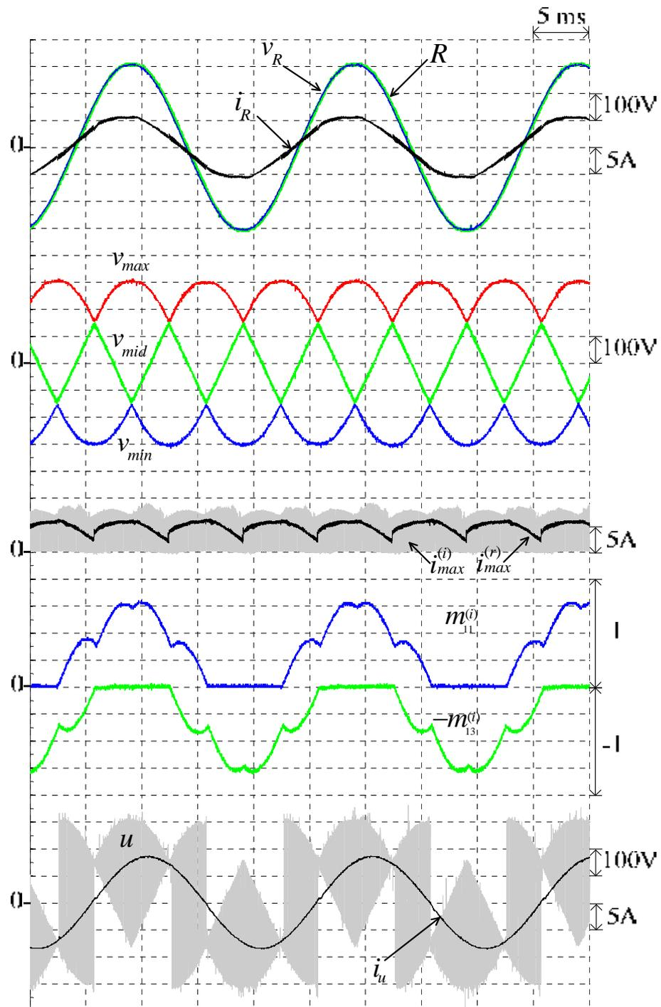
Figure 5.24 Measured waveforms of the prototyped S3L-BTB converter without input power factor compensation at ( $M = 0.7, f_o = 50 \text{ Hz}, k_1 = 0$ )
