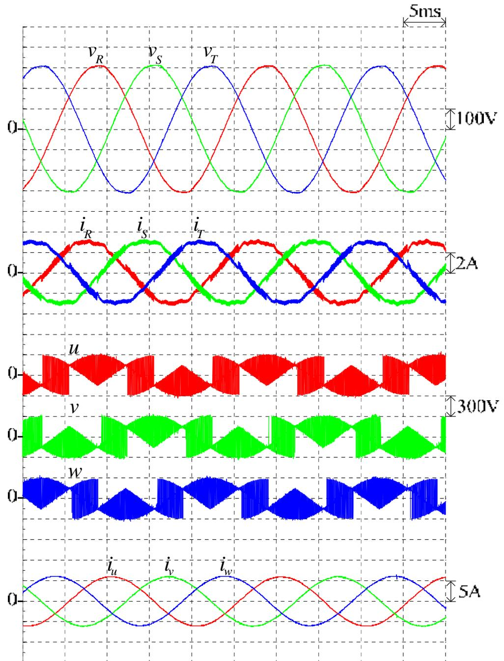
Figure 5.15 Measured input-output waveforms of the prototyped S3L-BTB converter under output voltage variation at ( $M = 0.5, f_o = 50$  Hz)
