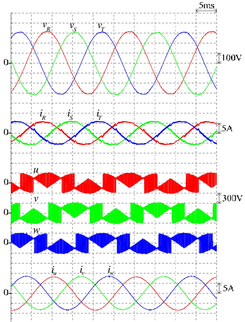
Figure 5.29 Measured input-output waveforms of the prototyped S3L-BTB converter with leading input power factor compensation at ( $M = 0.7$ ,  $f_o = 50$  Hz,  $k_1 = -3.3$ )
