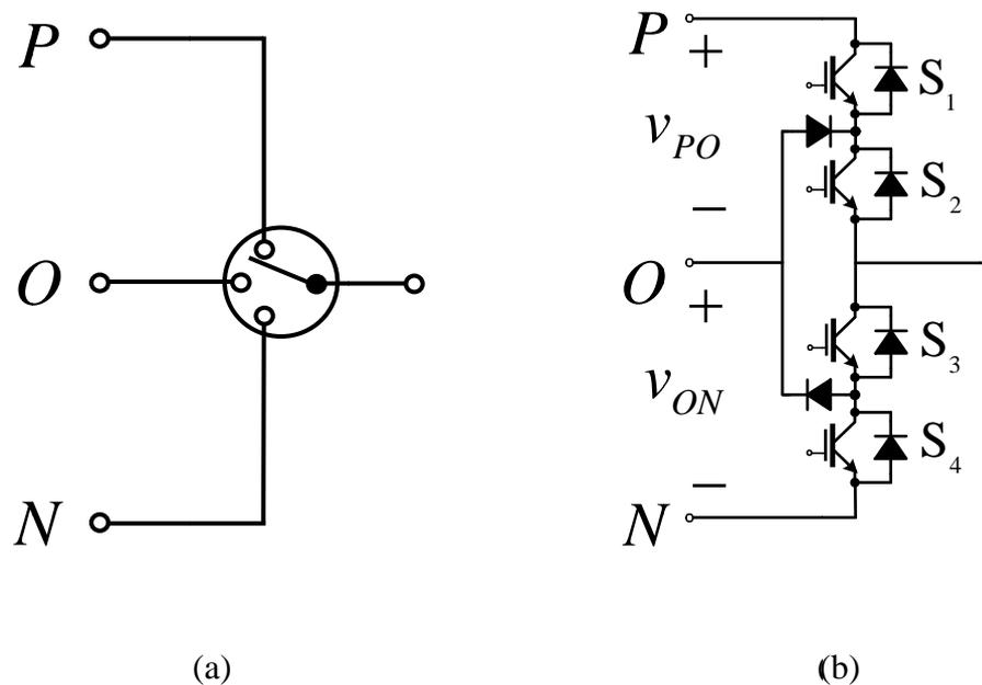
Figure 3.1 Single-phase NPC three-level converter topology.
