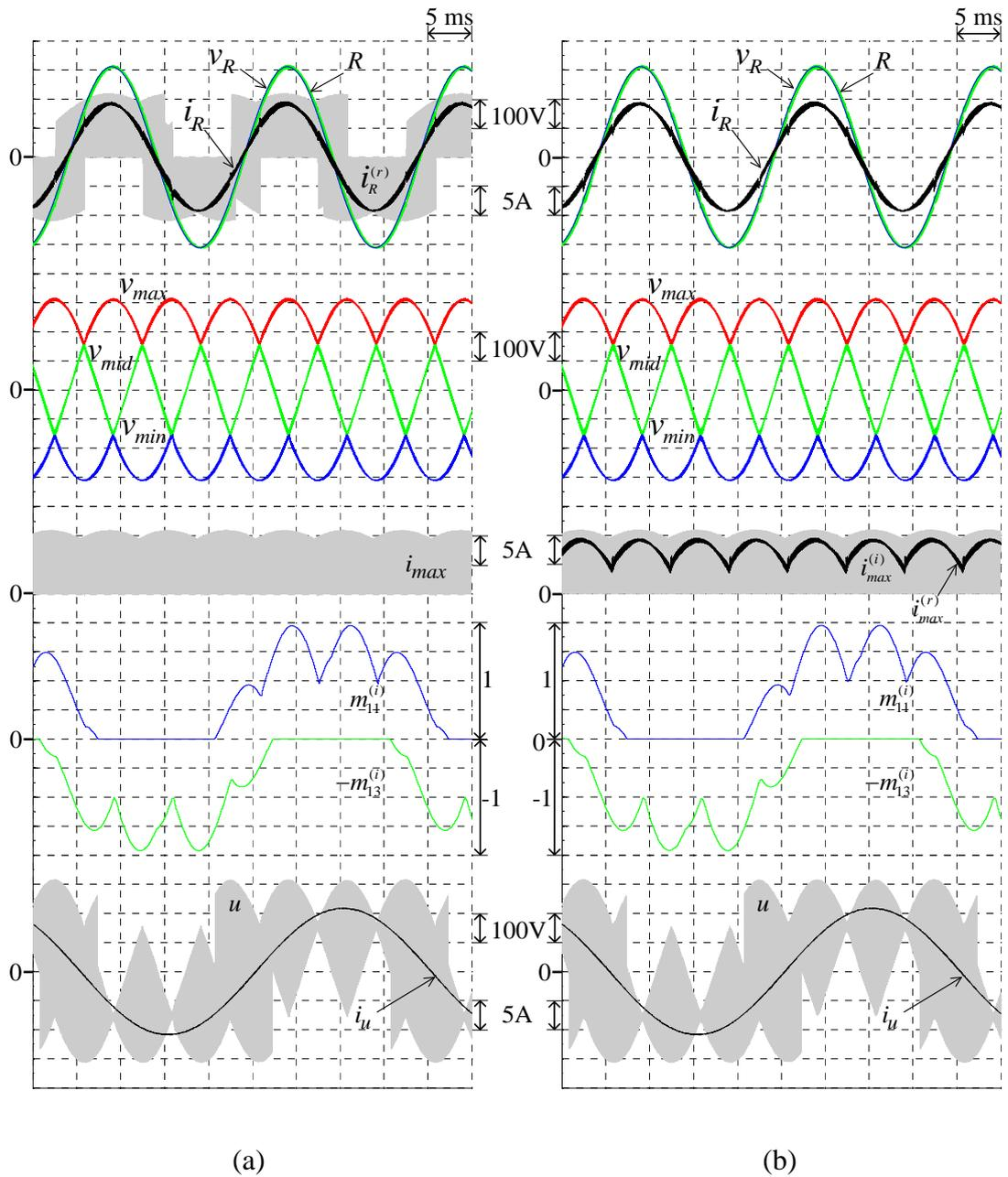
Figure 4.9 External and internal waveforms of the proposed 3L-BTB converters under output frequency variation ( $M = 0.86, f_o = 25$  Hz) (a) 3L-IMC (b) S3L-BTB converter
