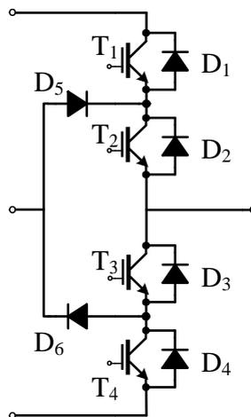
Figure 4.30 A three-level neutral-point-clamped structure used in loss evaluation
