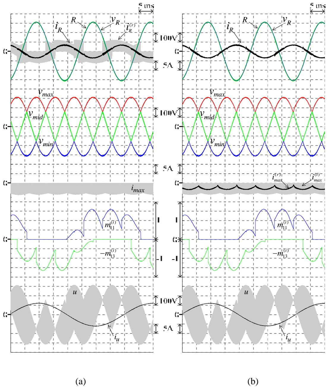
Figure 4.27 External and internal waveforms of the proposed 3L-BTB converters operating at unity input power factor under regenerative mode ( $M = 0.7$ ,  $f_o = 25$  Hz,  $k_1 = 12$ ) (a) 3L-IMC (b) S3L-BTB converter
