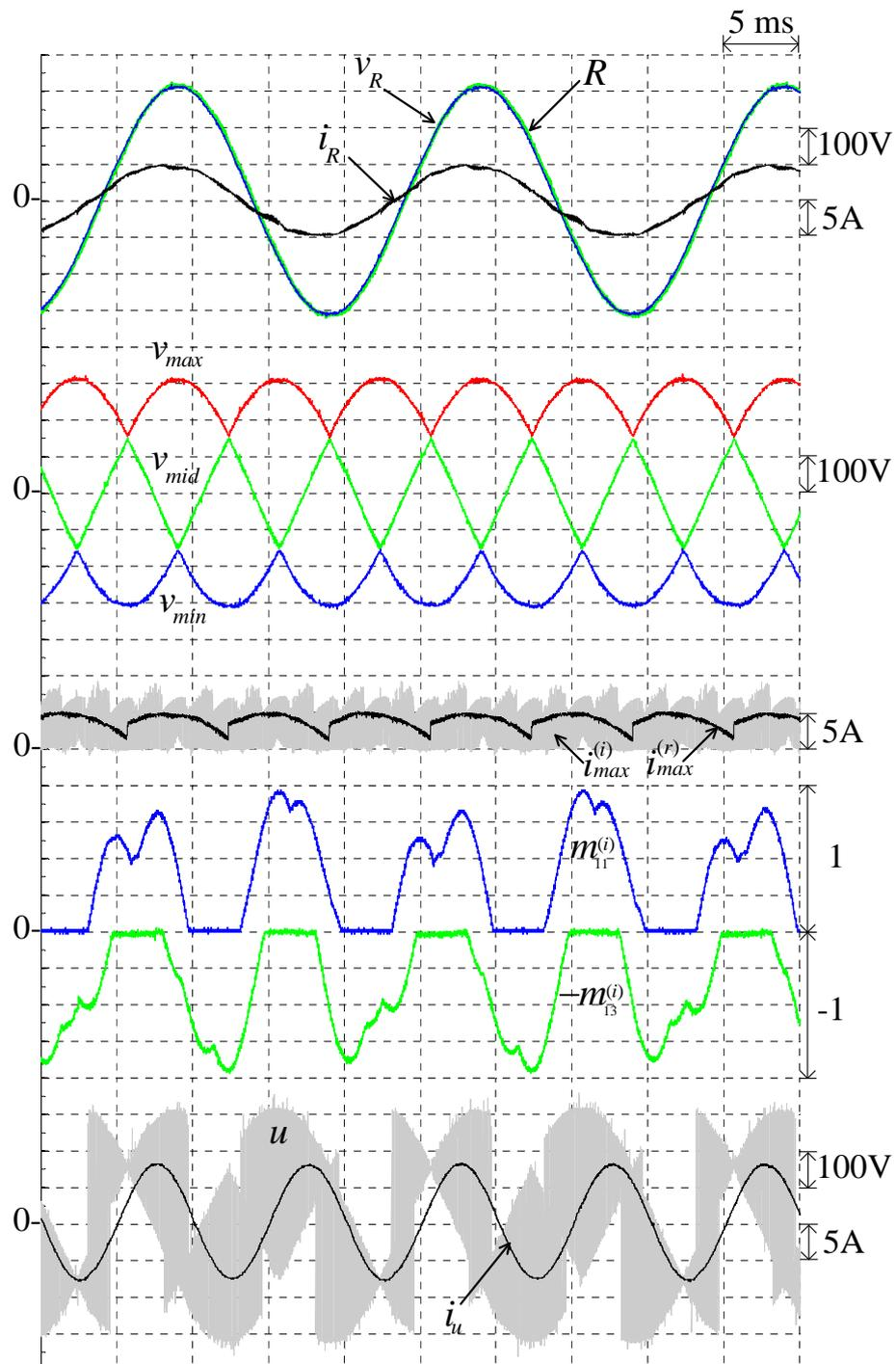
Figure 5.22 Measured waveforms of the prototyped S3L-BTB converter under output frequency variation at ( $M = 0.86, f_o = 100$  Hz)
