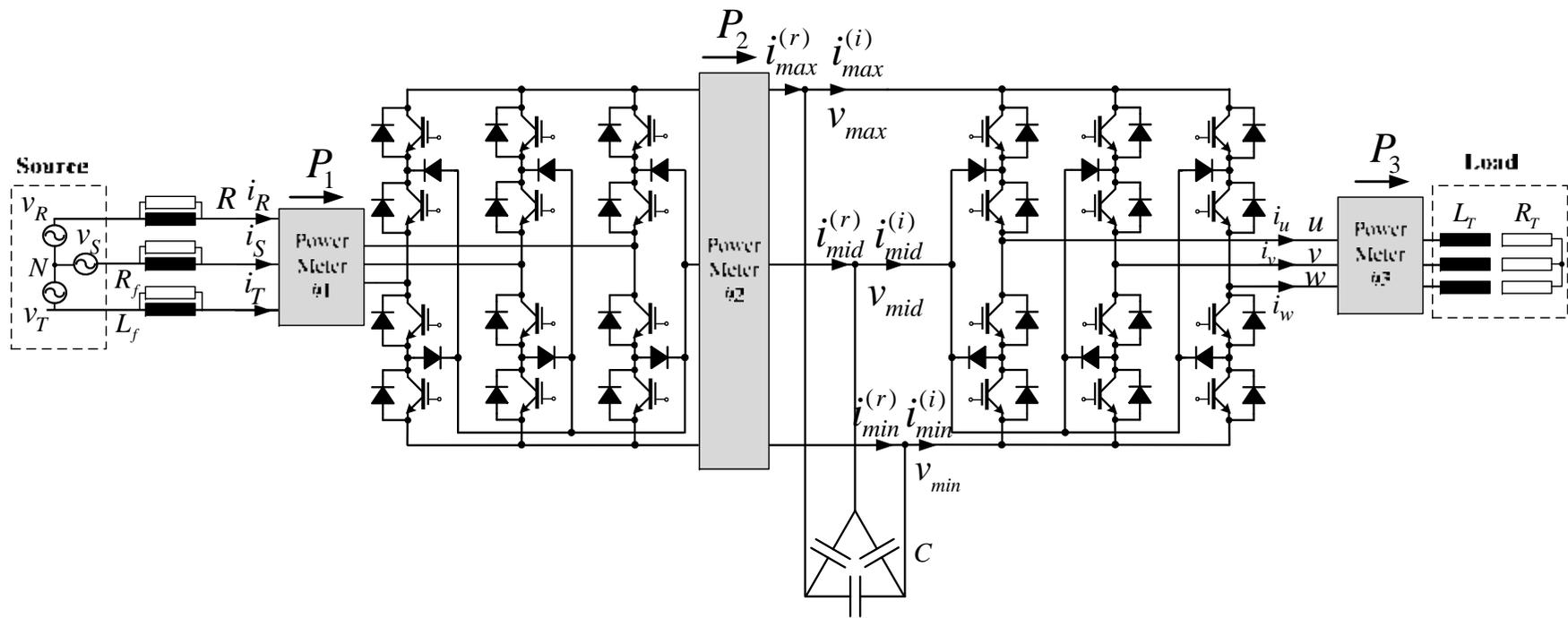
Figure 5.12 Schematic of the experimental setup for testing of the S3L-BTB converter.
