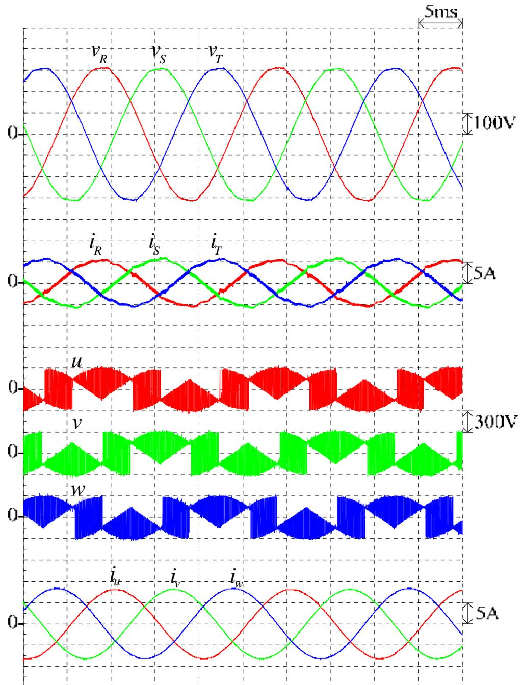
Figure 5.25 Measured input-output waveforms of the prototyped S3L-BTB converter with unity input power factor compensation at ( $M = 0.7$ ,  $f_o = 50$  Hz,  $k_1 = 5$ )
