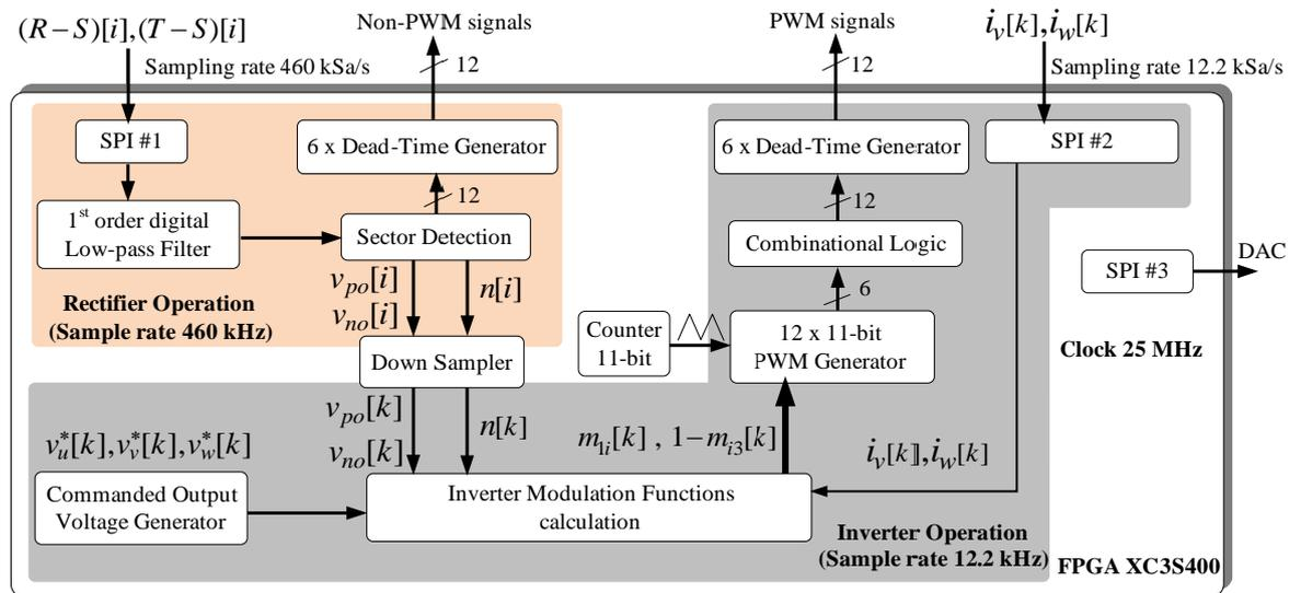
Figure 5.8 Hardware Modules synthesized and implemented on the FPGA.
