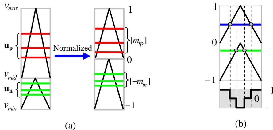
Figure 2.4 Double-carrier-based PWM for matrix converters. (a) two reference voltages and their normalization (b) switching signal for one phase.
