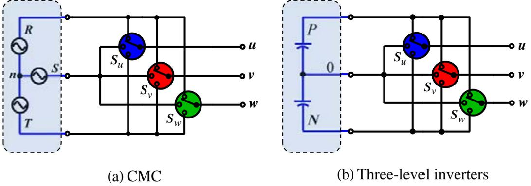
Figure 2.2 Similarity between the CMC and the three-level inverter.
