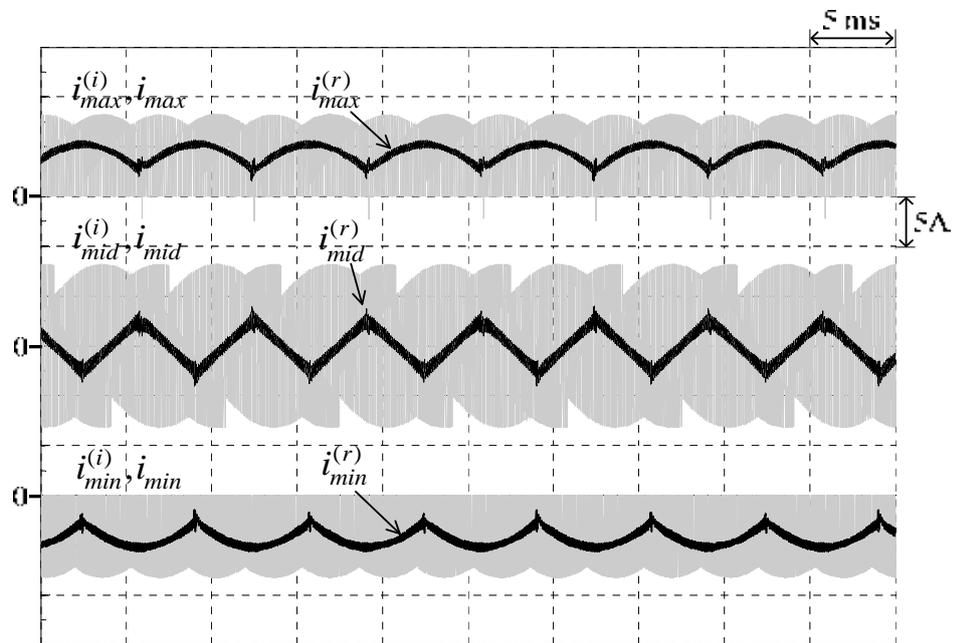
Figure 4.21 Simulated dc-link currents of the proposed 3L-BTB converters with unity input power factor under condition ( $M = 0.7, f_o = 50 \text{ Hz}, k_1 = 5$ )
