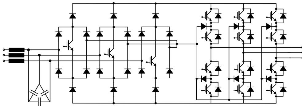
Figure 1.5 The three-level unidirectional indirect matrix converter (USMC3) topology
