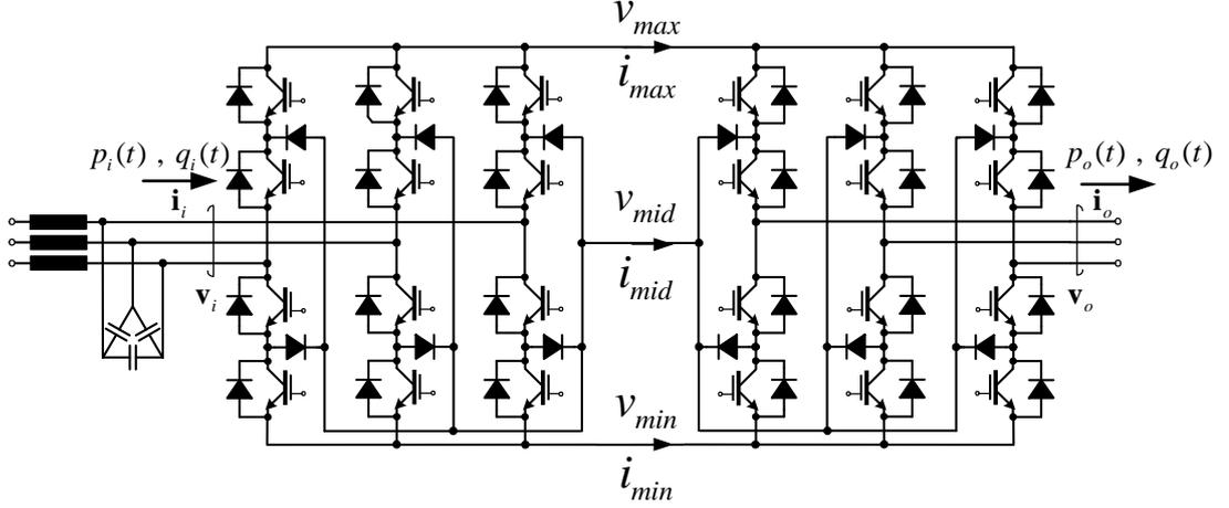
Figure 3.7 Definitions of variables in the 3L-IMC topology.
