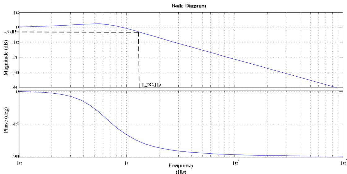
Figure 5.5 Frequency response of the designed input filter of the system
