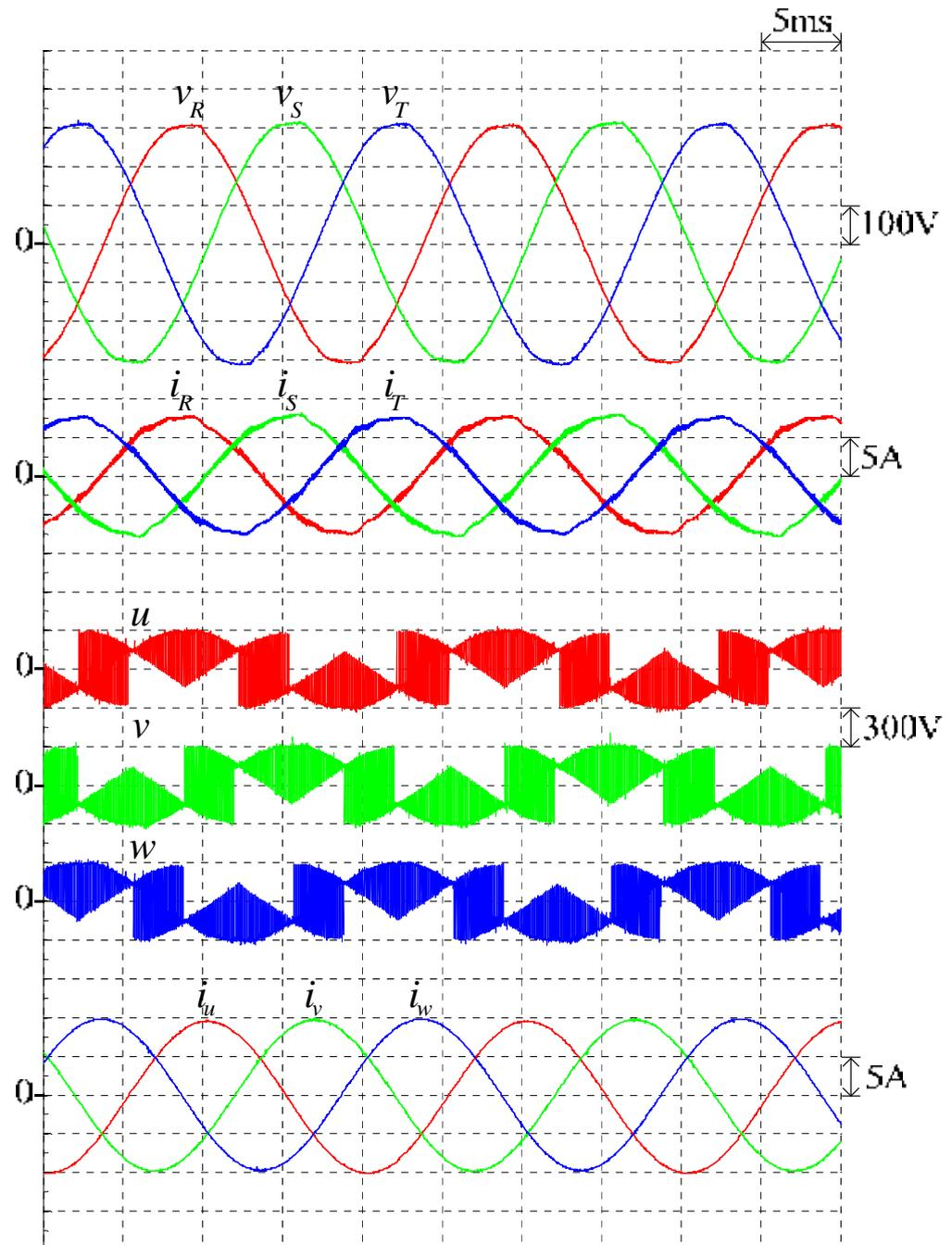
Figure 5.17 Measured input-output waveforms of the prototyped S3L-BTB converter under output voltage variation at ( $M = 0.86, f_o = 50$  Hz)
