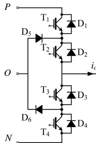
Figure A.1 A three-level neutral-point-clamped structure
