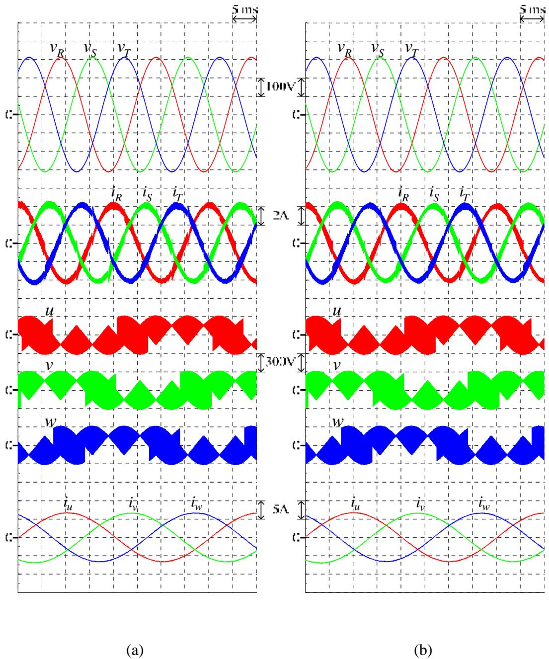
Figure 4.24 Simulated input-output waveforms of the proposed 3L-BTB converters operating under regenerative mode ( $M = 0.7$ ,  $f_o = 25$  Hz,  $k_1 = 0$ ) (a) 3L-IMC (b) S3L-BTB converter
