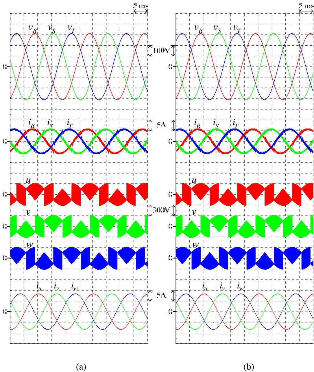
Figure 4.18 Simulated input-output waveforms of the proposed 3L-BTB converters with leading input power factor ( $M = 0.7$ ,  $f_o = 50$  Hz,  $k_1 = -3.3$ ) (a) 3L-IMC (b) S3L-BTB converter
