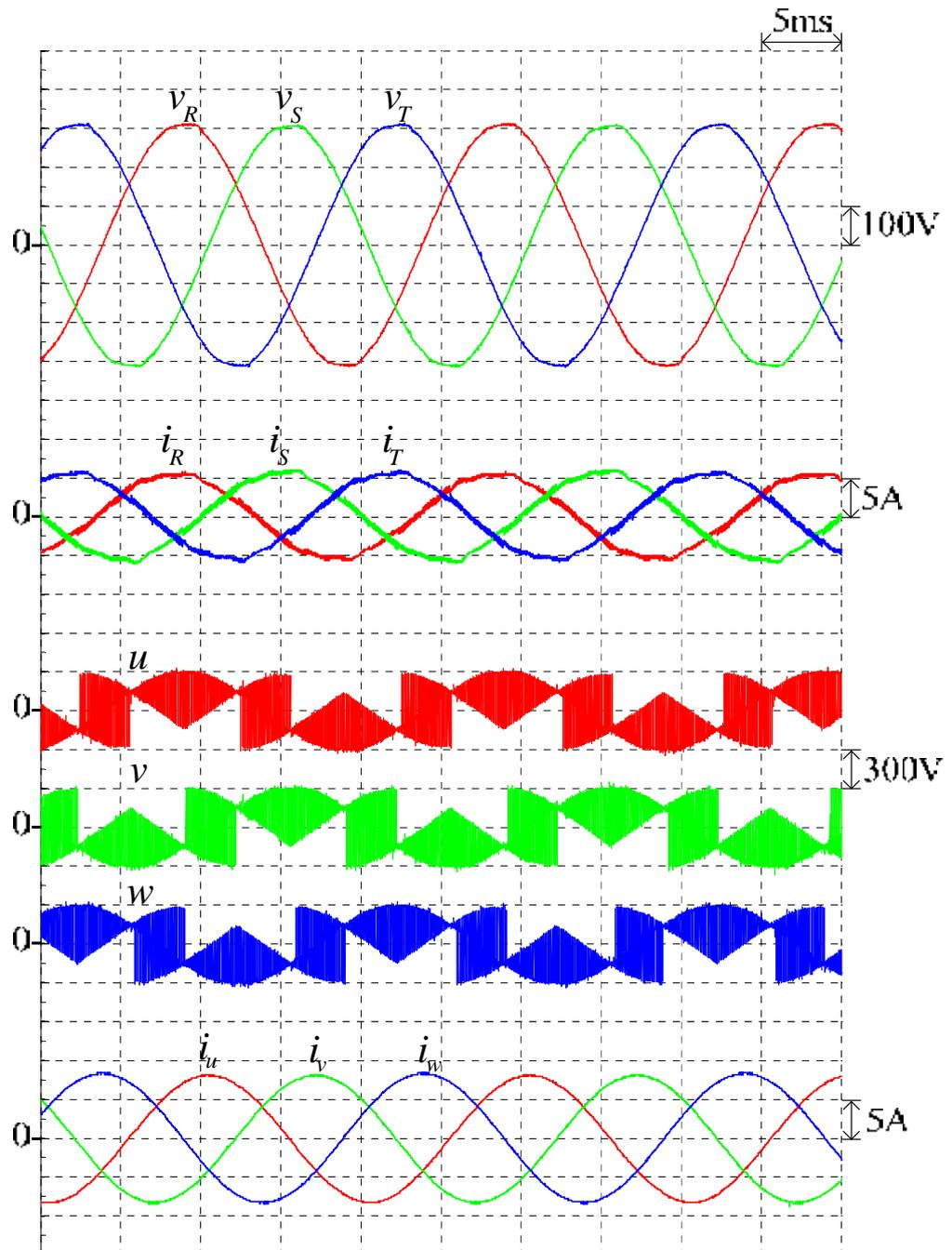
Figure 5.23 Measured input-output waveforms of the prototyped S3L-BTB converter without input power factor compensation at ( $M = 0.7, f_o = 50 \text{ Hz}, k_1 = 0$ )
