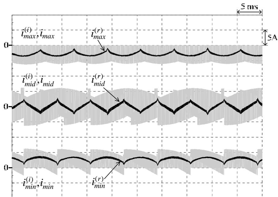
Figure 4.29 Simulated dc-link currents of the proposed 3L-BTB converters operating at unity input power factor under regenerative mode at ( $M = 0.7, f_o = 25 \text{ Hz}, k_1 = 12$ )
