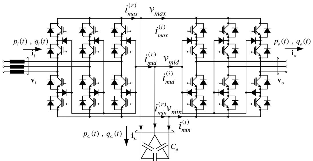
Figure 3.8 Definitions of variables in the S3L-BTB converter topology.
