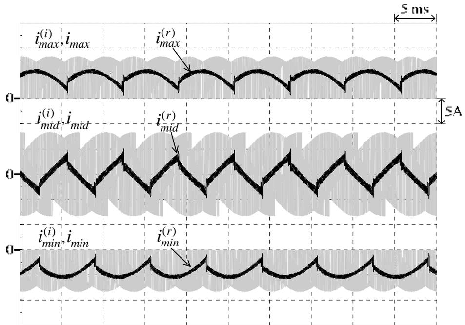
Figure 4.20 Simulated dc-link currents of the proposed 3L-BTB converters without input power factor compensation under condition ( $M = 0.7, f_o = 50 \text{ Hz}, k_1 = 0$ )
