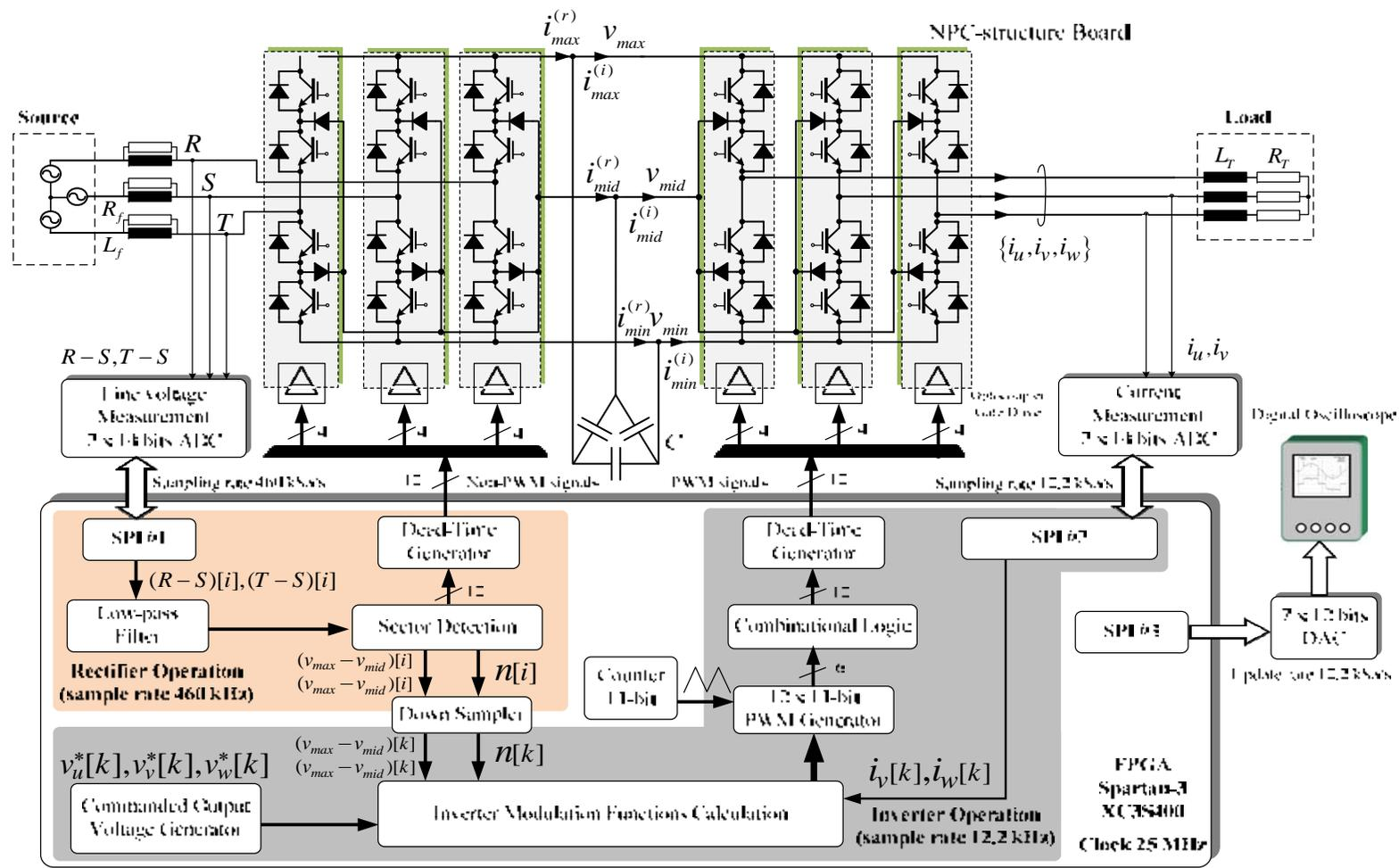
Figure 5.1 Schematic of laboratory prototype including functional diagram of the controller implemented on a FPGA.
