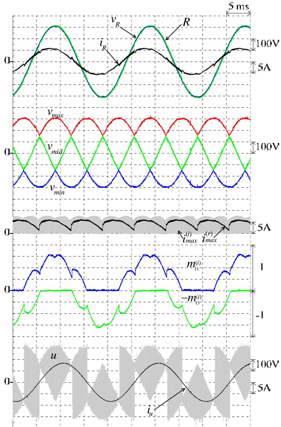
Figure 5.30 Measured waveforms of the prototyped S3L-BTB converter with leading power factor compensation at ( $M = 0.7, f_o = 50 \text{ Hz}, k_1 = -3.3$ )
