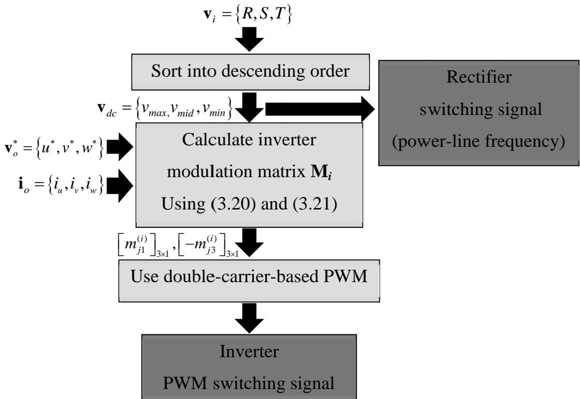
Figure 3.6 Flow chart of the modulation strategy for the proposed 3L-BTB converters
