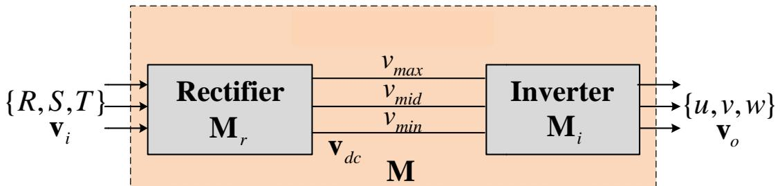
Figure 3.5 Three-level indirect modulation functions for the proposed 3L-IMC and S3L-BTB converters
