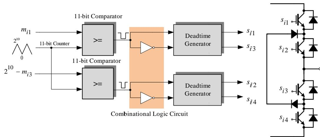
Figure 5.11 Simplified diagram of double-carrier-based PWM and the combinational logic circuit for generating the gate drive signals.
