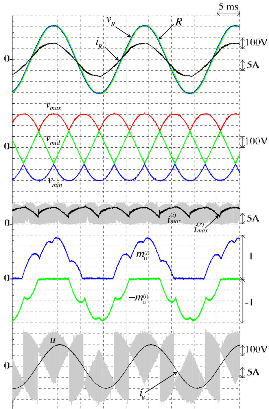
Figure 5.18 Measured waveforms of the prototyped S3L-BTB converter under output voltage variation at ( $M = 0.86, f_o = 50$  Hz)
