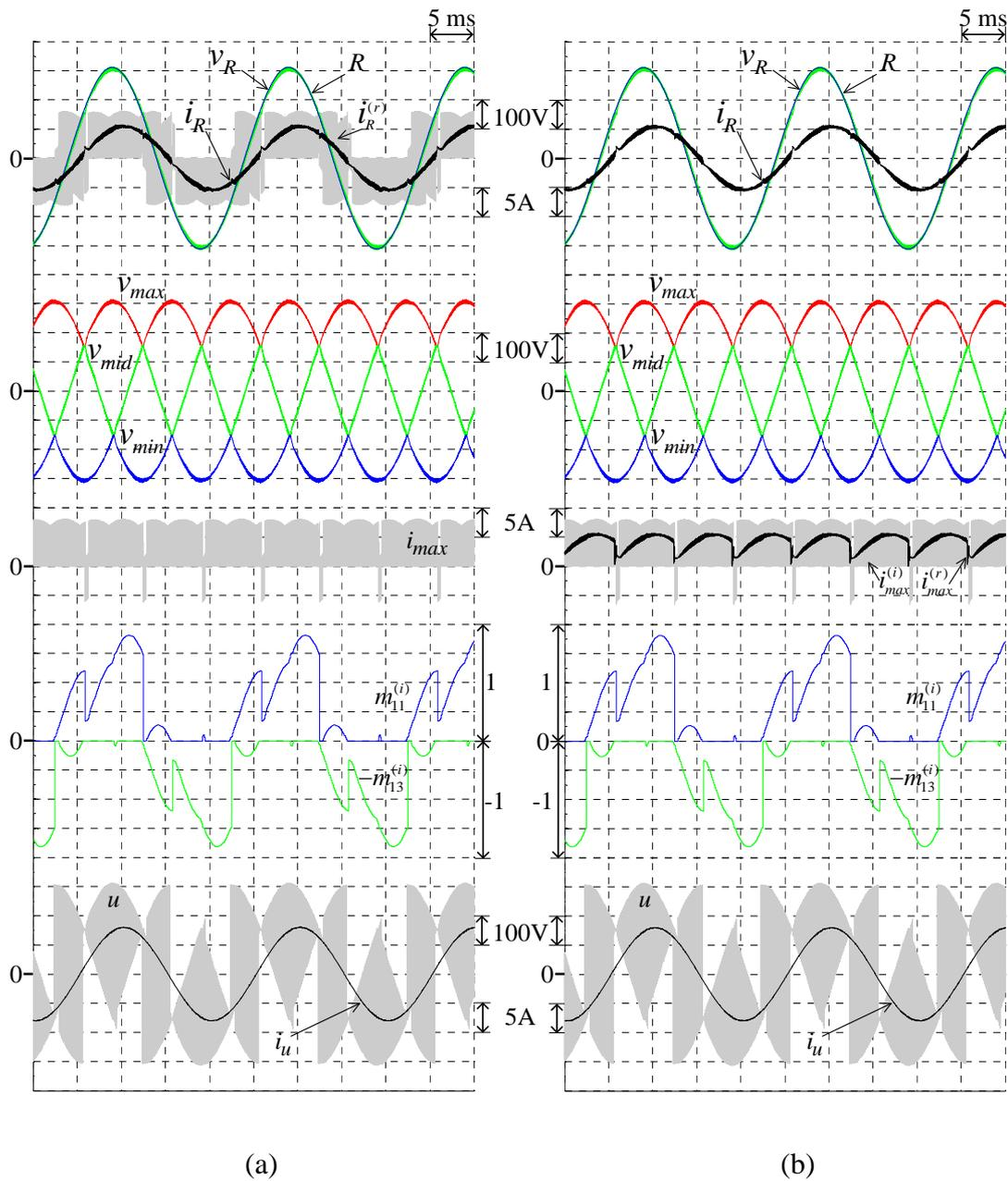
Figure 4.17 External and internal waveforms of the proposed 3L-BTB converters with lagging input power factor ( $M = 0.7$ ,  $f_o = 50$  Hz,  $k_1 = 15$ ) (a) 3L-IMC (b) S3L-BTB converter
