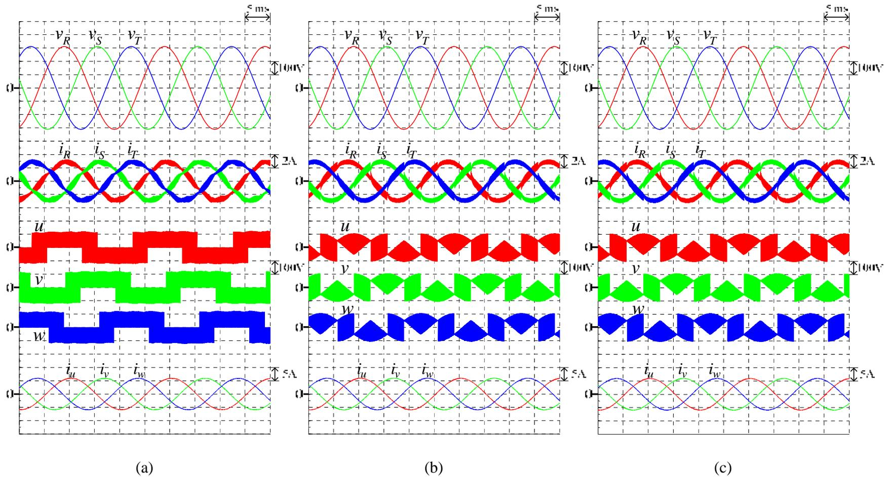
Figure 4.2 Simulated input-output waveforms of the 3L-BTB converters working under condition 1 ( $M = 0.5, f_o = 50$  Hz)
