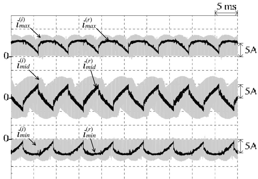
Figure 5.34 Measured dc-link current waveforms of the prototyped S3L-BTB converter with leading input power factor compensation at ( $M = 0.7, f_o = 50$  Hz,  $k_1 = -3.3$ )
