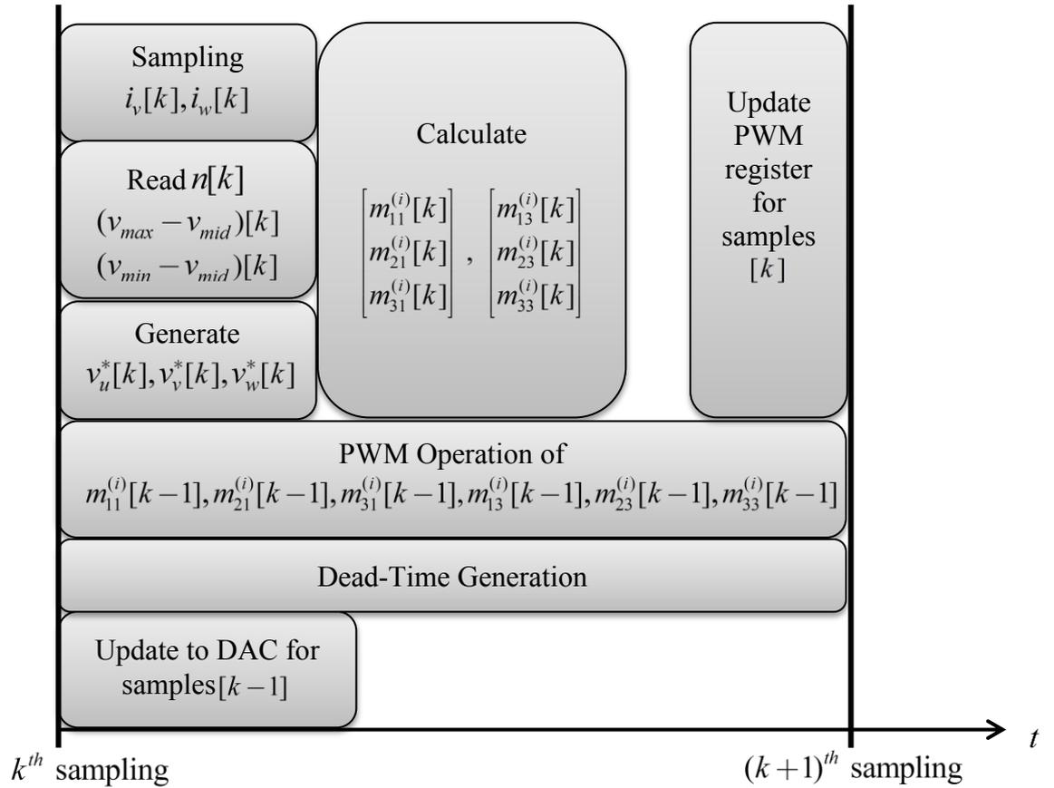
Figure 5.10 Timing diagram of the inverter operation implemented on the FPGA
