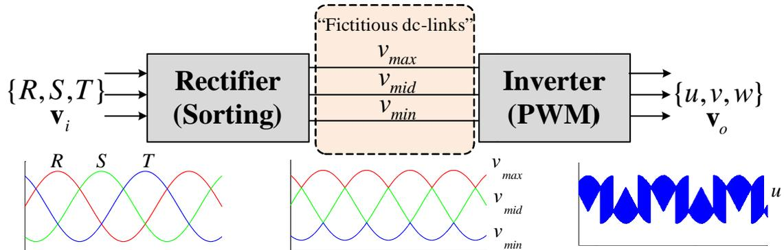
Figure 2.6 Three-level indirect modulation strategy derived from double-carrier-based PWM.
