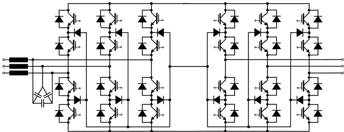
Figure 3.3 Three-level indirect matrix converter (3L-IMC).
