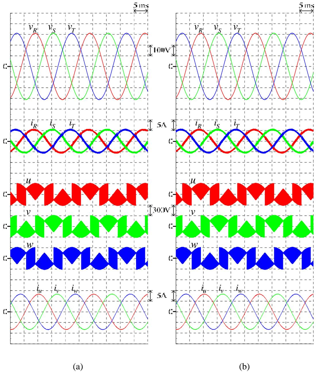
Figure 4.12 Simulated input-output waveforms of the proposed 3L-BTB converters without input power factor compensation ( $M = 0.7$ ,  $f_o = 50$  Hz,  $k_1 = 0$ ) (a) 3L-IMC (b) S3L-BTB converter
