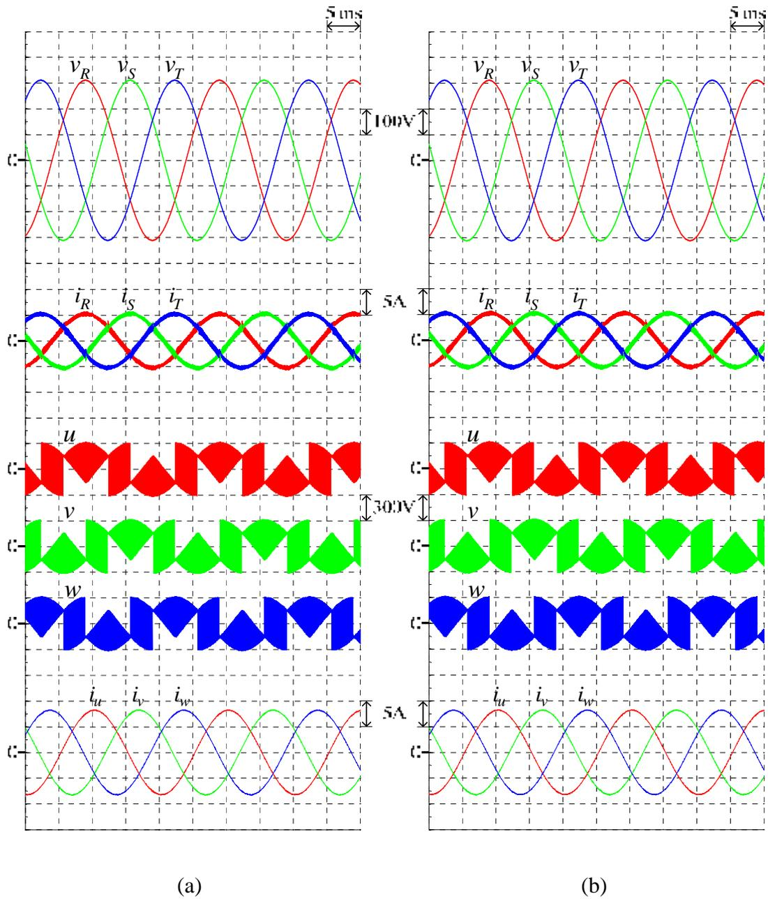
Figure 4.14 Simulated input-output waveforms of the proposed 3L-BTB converters with unity input power factor ( $M = 0.7$ ,  $f_o = 50$  Hz,  $k_1 = 5$ ) (a) 3L-IMC (b) S3L-BTB converter
