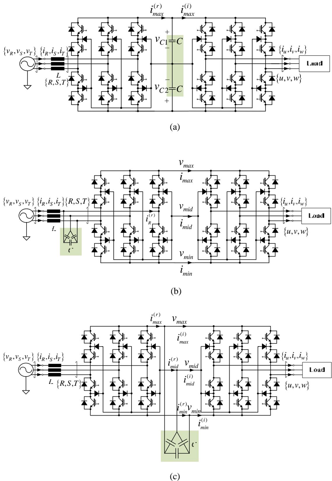
Figure 4.1 Three-level BTB converter topologies. (a) conventional 3L-BTB converter
