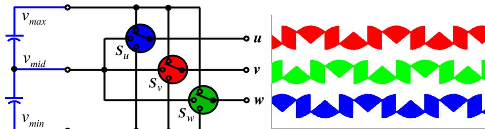
Figure 2.5 Conceptual diagram of the inverter stage with the unidirectional dc-link voltages and its generated output PWM voltages
