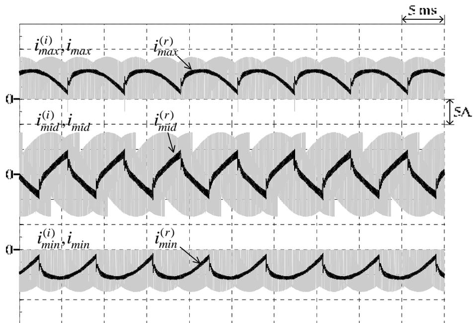
Figure 4.23 Simulated dc-link currents of the proposed 3L-BTB converters with leading input power factor under condition ( $M = 0.7, f_o = 50 \text{ Hz}, k_1 = -3.3$ )
