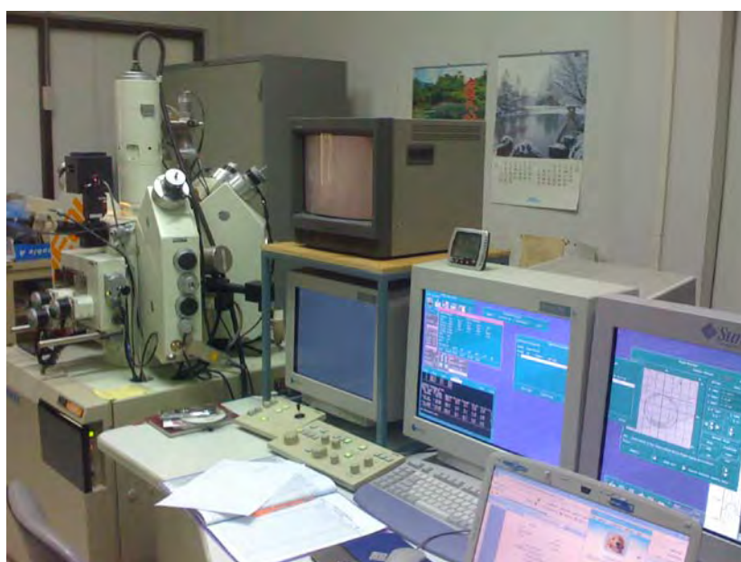
Figure 1.3 Electron Probe Micro-Analyzer (EPMA) (JEOL model JXA-8100) based at Department of Geology, Faculty of Science, Chulalongkorn University applied for analysis of mineral chemistry.
