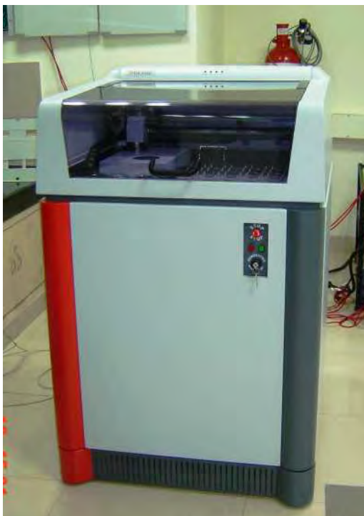
Figure 1.4 X-Ray Fluorescence Spectrometry (Model Bruker axs S-4 Pioneer) based at Faculty of Science, Chulalongkorn University applied for whole-rock analysis.
