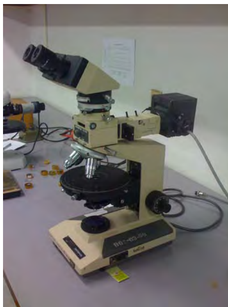
Figure 1.2 Polarizing Microscope based at the Geology Department, Chulalongkorn University used for petrographic works.
