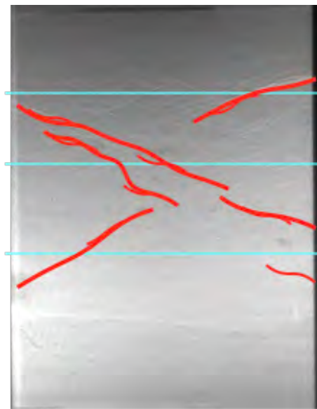
Figure 5.5 shows the third state of fracture development: fractures observed (red), permeability increases.
