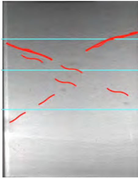
Figure 5.4 shows the third state of fracture development: cracks connection (red).
