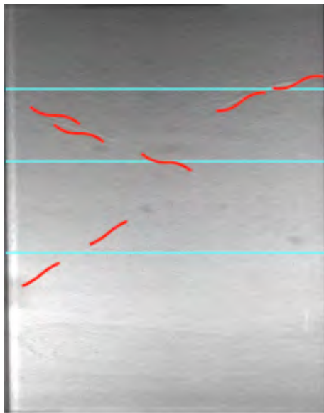
Figure 5.3 shows the second state of fracture development: growth of cracks (red).
