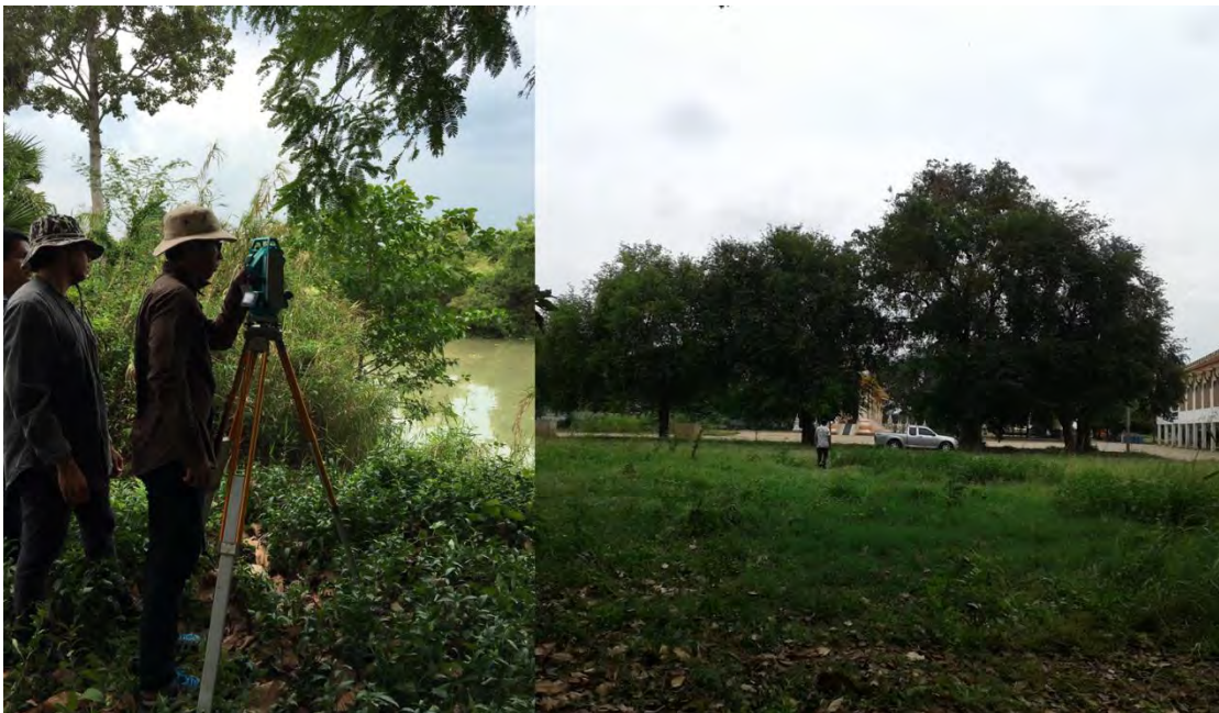
Figure 8. Total station survey for creating river bank height profile
