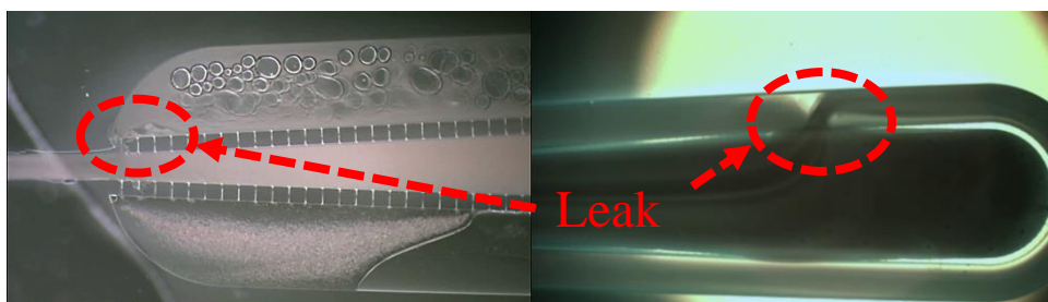
Figure 21 Damage at micro capillaries wall
