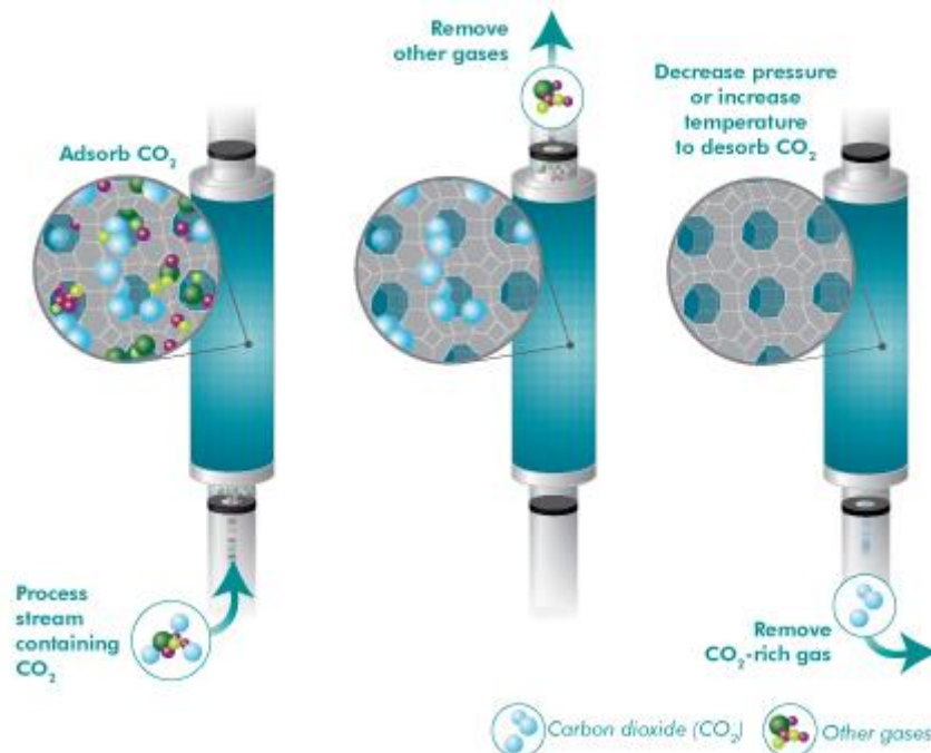
Fig. 2.6 Basic steps of pressure and vacuum swing adsorption-desorption cycle [29].
