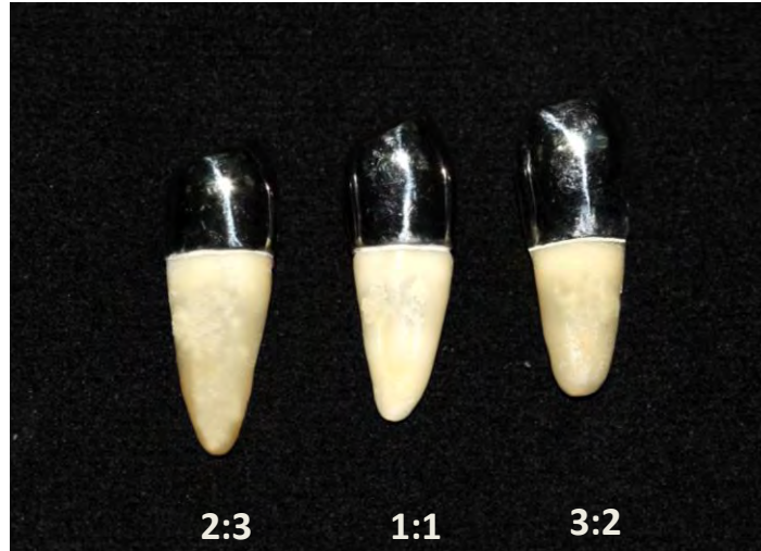
Figure 6 Specimens with three different core to fiber post length ratios.
