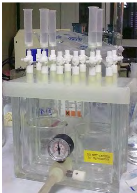
Figure 3.5 Vacuum manifold used with chelating disk cartridge
