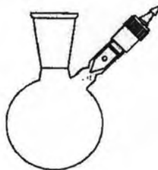
Figure 3.2 Round-bottomed Schlenk flask.
