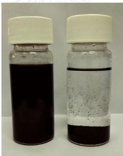
Figure 4.5 The difference of dispersive ability between CNT (left) and O-CNT (right) in octanol within 2 days
