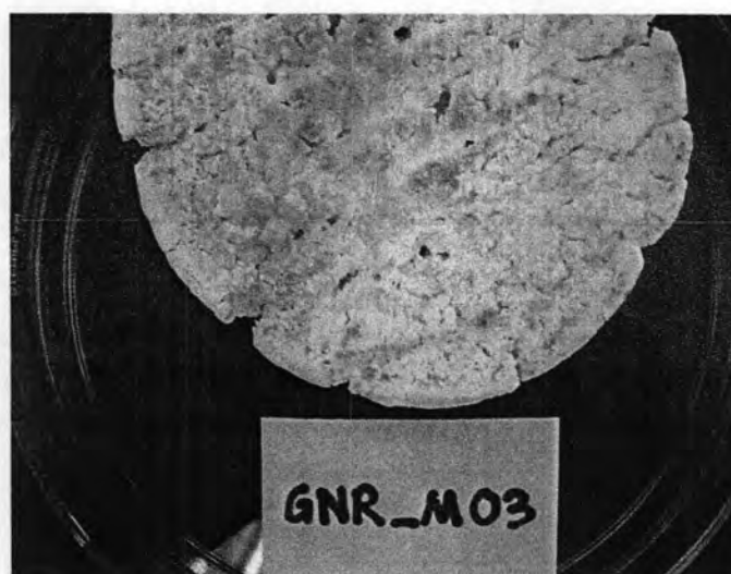
Figure 4.8 Gross graft product obtained from microwave induced graft copolymerization of MMA onto NR at 100 W for 20 min (%GNR = 65.2).
