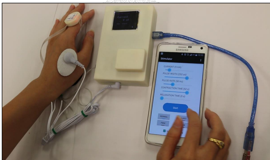
Figure 7: The prototype model for the tremor detection and suppression device (Parkinson's glove)
