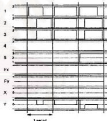
Fig.4 Valve diagram of the PWM technique. The number 1-5 is valve number, F_x and F_y are a direction of force act on piston, X and Y are the motion of cylinder present only direction.
