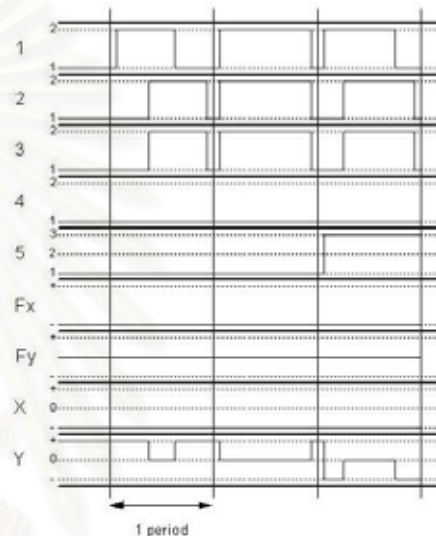
Fig.3 Valve diagram of the PWM technique. The figure 1-5 are valve number, F_x and F_y are a direction of force act on piston, X and Y are the motion of cylinder present only direction.
