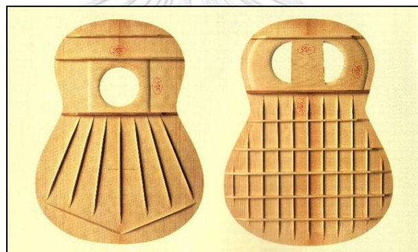
Figure 7: Bracing of Paul Fischer's guitar: Torres guitar style (left), lattice style (right)
