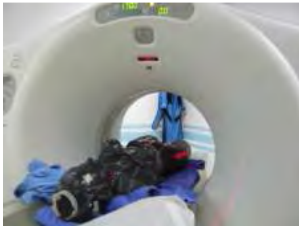
Figure 3.21 The Alderson Rando phantom scanning.
