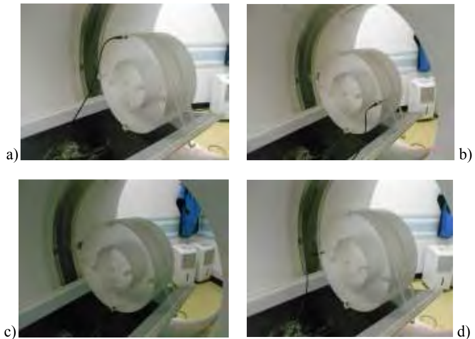
Fig. 3.15 The pencil ionization chamber at the peripheries of the body phantom.
