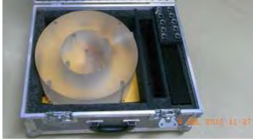
Fig. 3.7 The head and body PMMA phantom.
