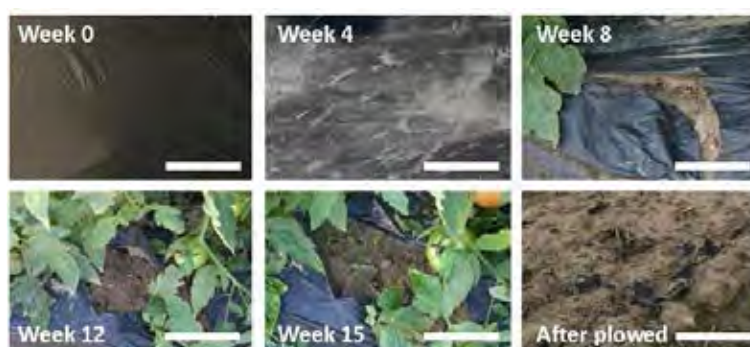
Figure 2.3 Pictures of the black biodegradable films during and after the growing season (bar length equals 5 cm).
