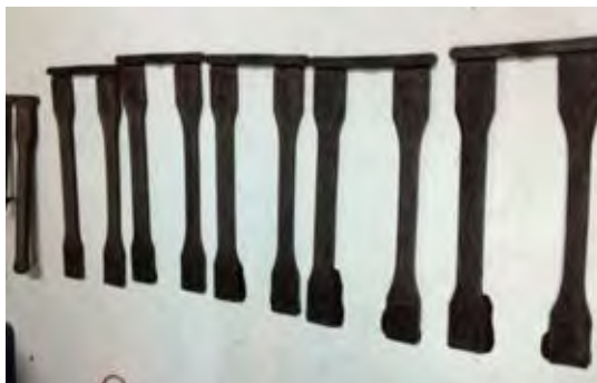
Figure 3.6 Dumbbell specimen for tensile testing.
