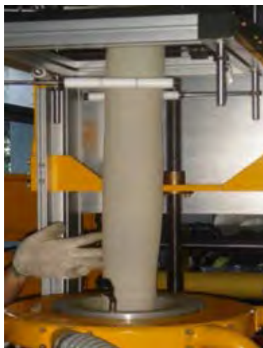
Figure 3.8 Preparation of bagasse/PLA composite films by using blown film extrusion.
