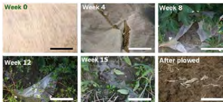
Figure 2.2 Pictures of the white biodegradable films during and after the growing season (Bar length equals 5 cm).
