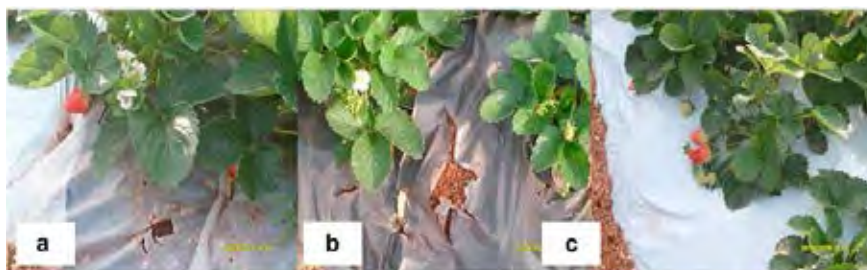
Figure 2.4 (a) white biodegradable film, (b) black biodegradable film, and (c) control polyethylene film after 5 weeks in contact with soil.
