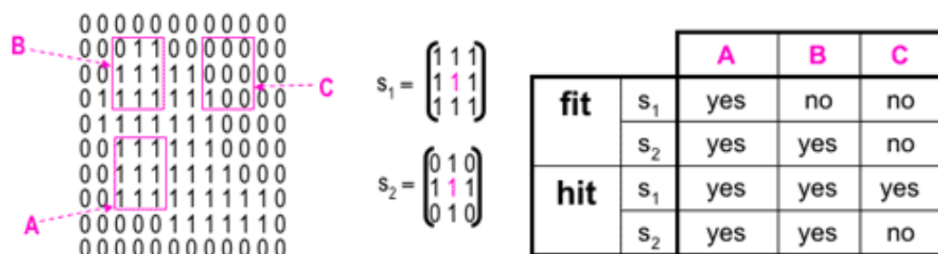
Figure 12. Examples of fitting and hitting of the structuring element s_1 and s_2
