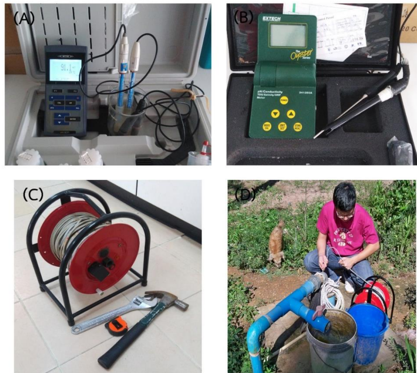
Figure 3.9 Equipment for parameters measurement in the field. (A) pH 3210 WTW meter for measuring pH and ORP. (B) 341350A-P Oyster Series meter for measuring EC, T and TDS. (C) Equipment for measuring water level. (D) Procedure of water level measurement.
