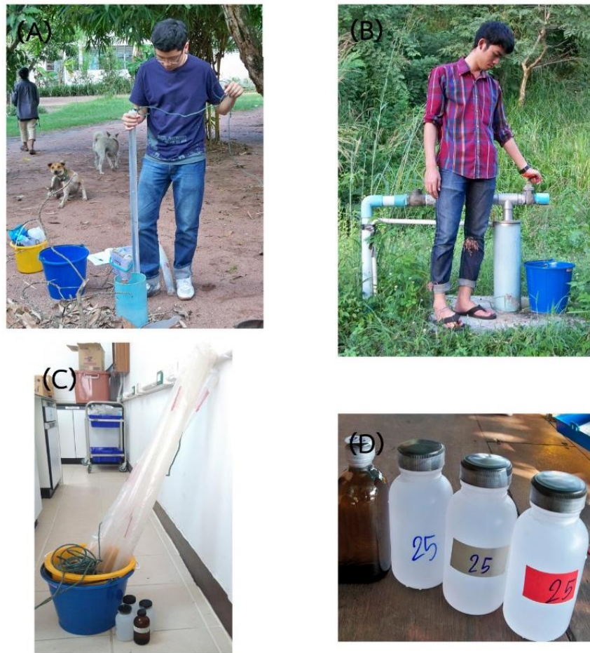
Figure 3.8 Groundwater well and equipment used in samples collecting (A) The open well, (B) The installed pump well, (C) Equipment for groundwater sampling and (D) Water samples in polyethylene bottles
