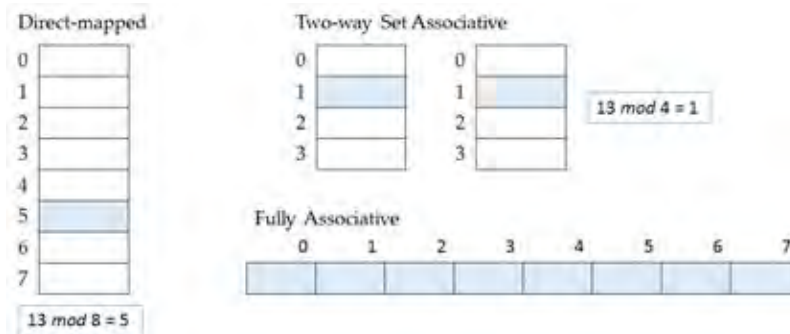
Figure 2.1: Three types of cache organizations. This is an example of the cache where block address 13 can be allocated in the gray area. In direct-mapped, 13 \bmod 8 = 5 ; the block should be located at location 5. In two-set associative cache, 13 \bmod 4 = 1 ; the block can be allocated at one of the two blocks at location 1. In fully-associative cache, a block can be allocated anywhere.
