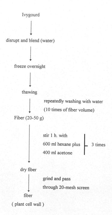
Figure 3 Steps in preparation of plant fiber.
