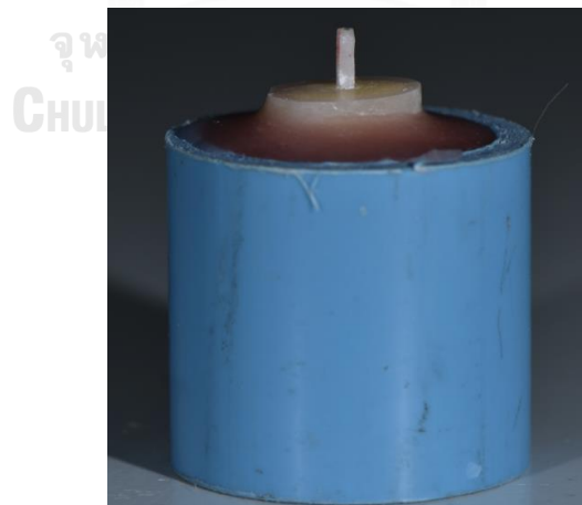
Figure 10. ZLS microbar cemented to dentin specimen
