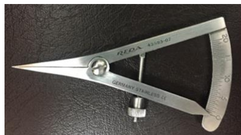
Figure 11 Caliper with 2 spikes for Static Two-Point discrimination and Moving Two-Point Discrimination test
