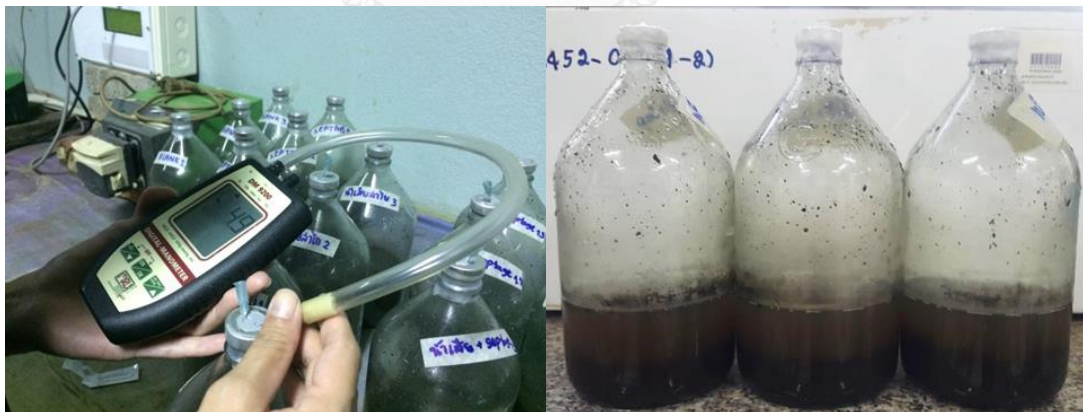
Figure 3.4 Modified BMP test
