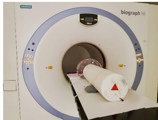
Figure 46 Positioning of IEC body phantom and scatter phantom for testing image quality of PET/CT system.
