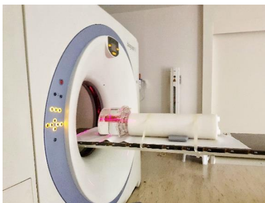
Figure 15 Positioning of IEC body phantom for testing image quality of PET/CT system.
