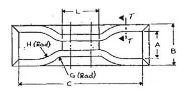
Figure 3.1 Schematic of tensile specimen
