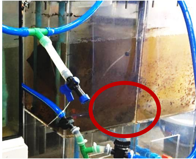
Figure 4.12. Solid sediments on tank floor of solid separating unit and biofilm formation
