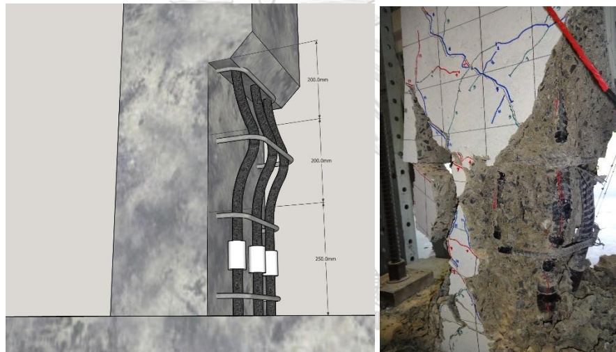
Figure 4.22 Plastic hinge length of MS1 column equal to 650 mm
