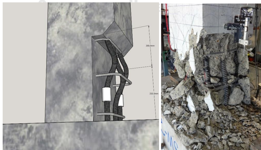
Figure 4.23 Plastic hinge length of MS2 column equal to 450 mm
