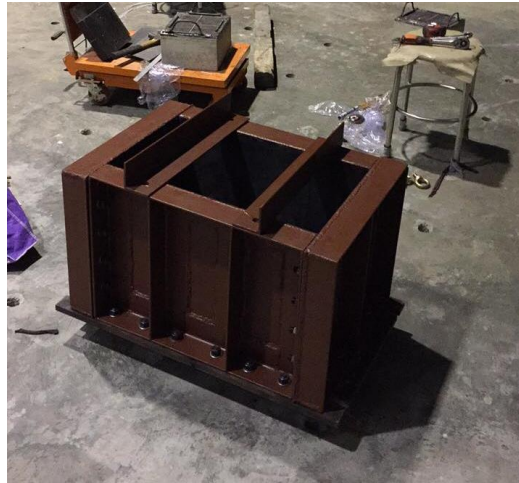
Figure 3.12 General view of ballast box apparatus
