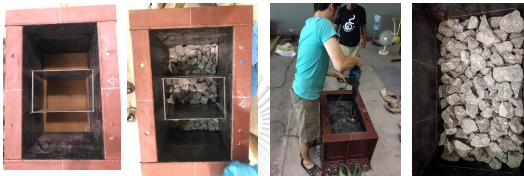
Figure 3.2 Visualizing appearance and placing of the ballast in the box.
