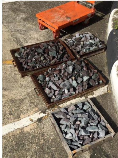
Figure 3.6 Visual appearance of ballast.
