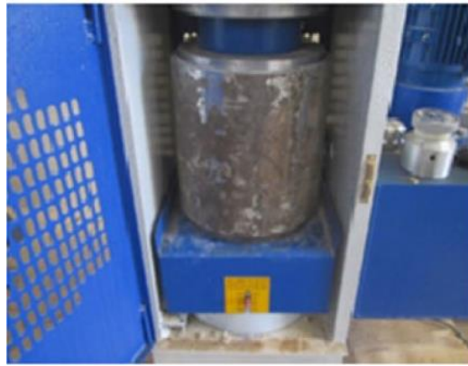
Figure 2.7 Crushing test apparatus (Koohmishi and Palassi, 2018)
