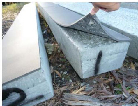
Figure 2.13 Under sleeper pads (Kaewunruen and Remennikov, 2015)
