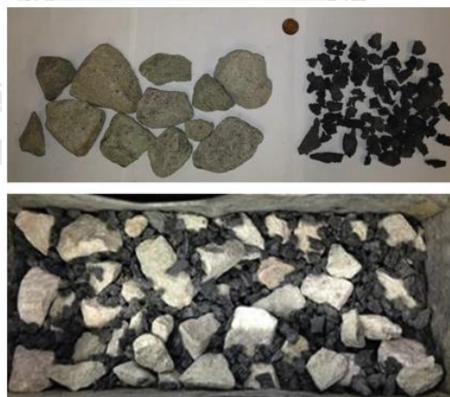
Figure 2.14 The ballast and crumb rubber material mixing in box apparatus (M. Sol-Sánchez et al., 2015).
