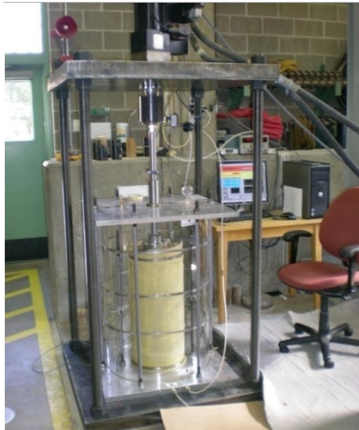
Figure 2.8 Large-Scale Cyclic Triaxial Test Equipment, Loading Machine, and Data Acquisition System (Ebrahimi et al., 2010)
